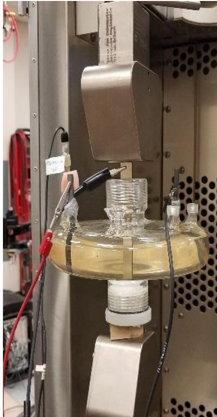
Figure 2.6 The mechanical-electrochemical setup includes a conventional three electrode configuration with a graphite rod as the counter electrode, a saturated calomel electrode with a Luggin capillary as the reference electrode, and a metallic ASTM tensile sample was the working electrode.
