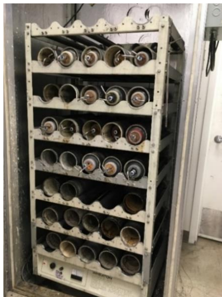
Figure 4-3. Thermostatic incubator equipped with rollers.
