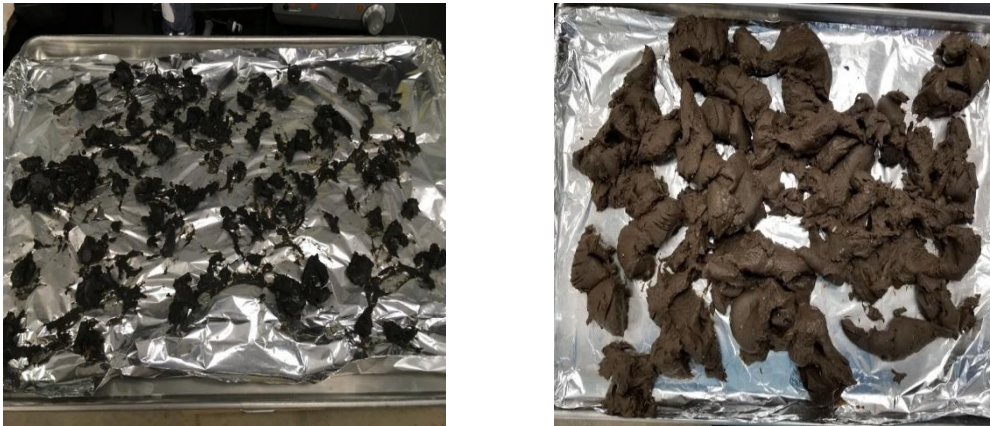
Figure 2-3. Air-dried and fresh sewage sludge.
