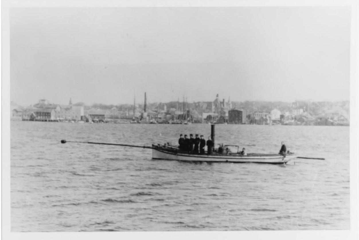
Figure 18. An early unidentified torpedo-bearing steam launch. Reprinted with permission of the Naval History and Heritage Command (NH 82827).
