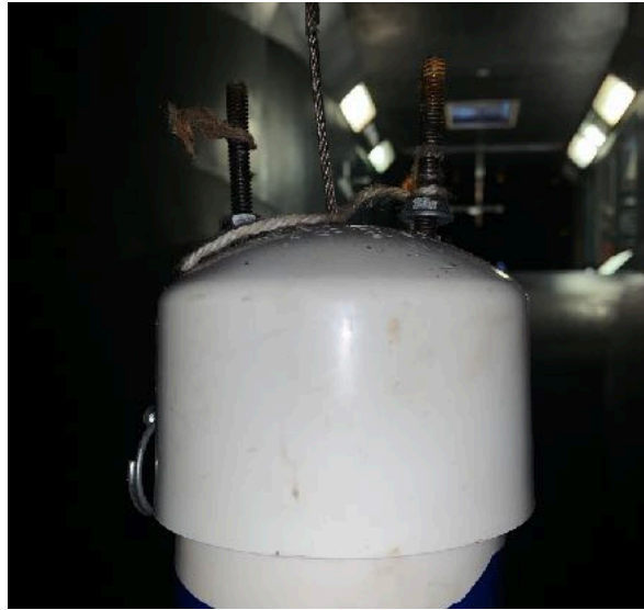
Figure 30: Selective Seeding System Ceiling Connection
