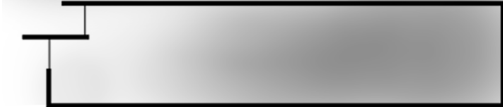
Clearstory Window for Daylighting
