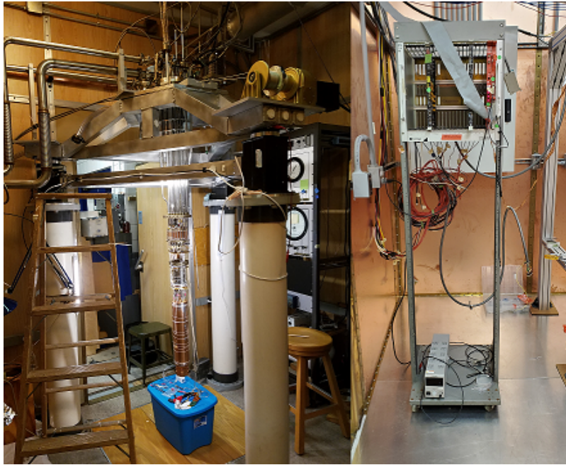
Figure 2.14: Dilution refrigerator disassembled (left) and example of front end readout electronics (right). The detector, inside a special housing and read out by cryogenic electronics, is installed in the dilution refrigerator at left. The cryogenic electronics are further read out by the electronics at room temperature, similar to those shown at right. The left photograph shows the Texas A&M University facility in 2016, and the right one is from a related Texas A&M University facility in 2020.
