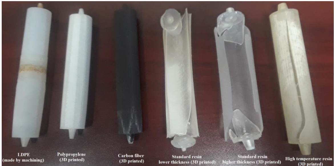
Figure 50. Different types of 3D printed floats along with the one made by machining
