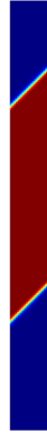
Figure 6.9 Liquid-vapor equilibrium with a flat but inclined interface ( \theta = 45^\circ ); Red: liquid phase; Blue: vapor phase.
