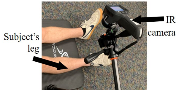
Figure 3.5: Proof of Concept experimental layout for supine subject
