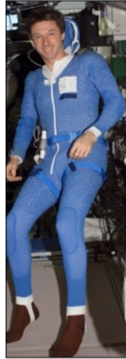
Figure 2.9: Russian Orlan LCG which includes a hood, with tubing covering the trunk, arms, thighs and portions of the neck and head. Reprinted from [17]
