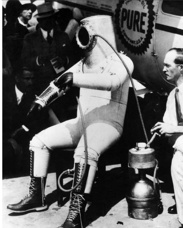
Figure 1.2: Wiley Post demonstrating his fully pressurized suit in front of Winnie Mae. Reprinted from [1]
