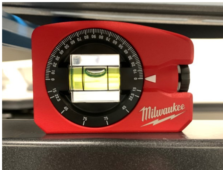
Figure 4.14: The Milwaukee 4 in Pocket Level will be attached to the center metal support bar of the tilt table through magnets, and will allow the operator to verify the tilt angle
