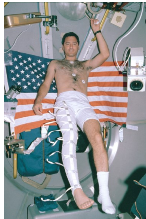
Figure 2.18: Astronaut Larry DeLucas wearing stocking plethysmograph on United States Micro-gravity Laboratory 1 (USML-1) (STS-50) in 1992. Reprinted from [62]
