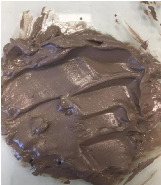
Figure 4.3 Consistency of a typical FFT cake sample at liquid limit
