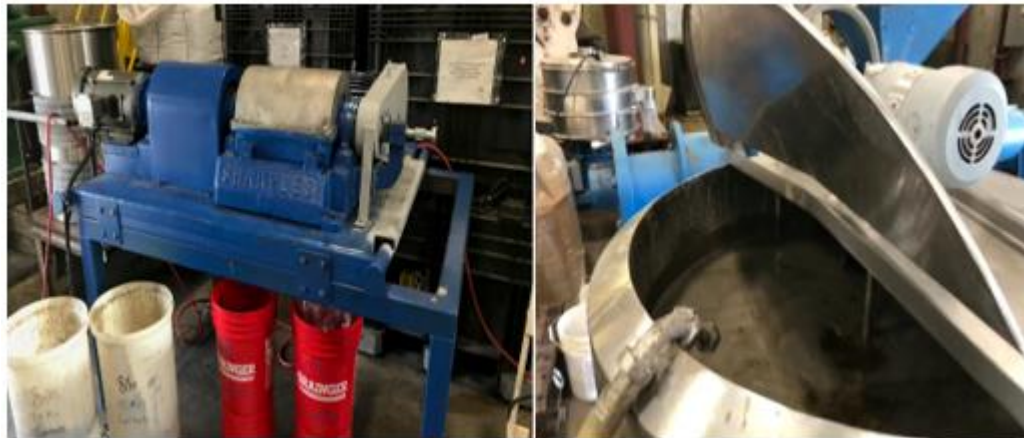
Figure 3.1 Pilot scale horizontal decanter centrifuge test study for dewatering FFTs
