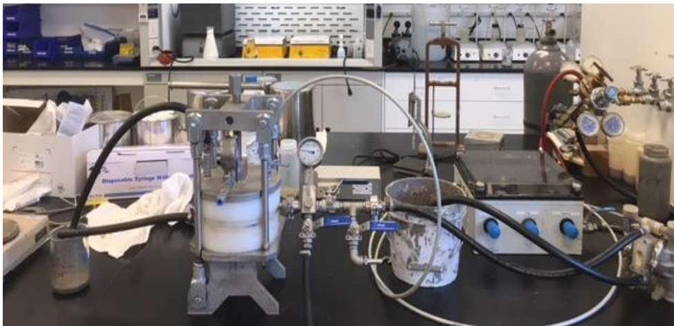
Figure 4.1 Pressure filtration test setup to dewater FFTs
