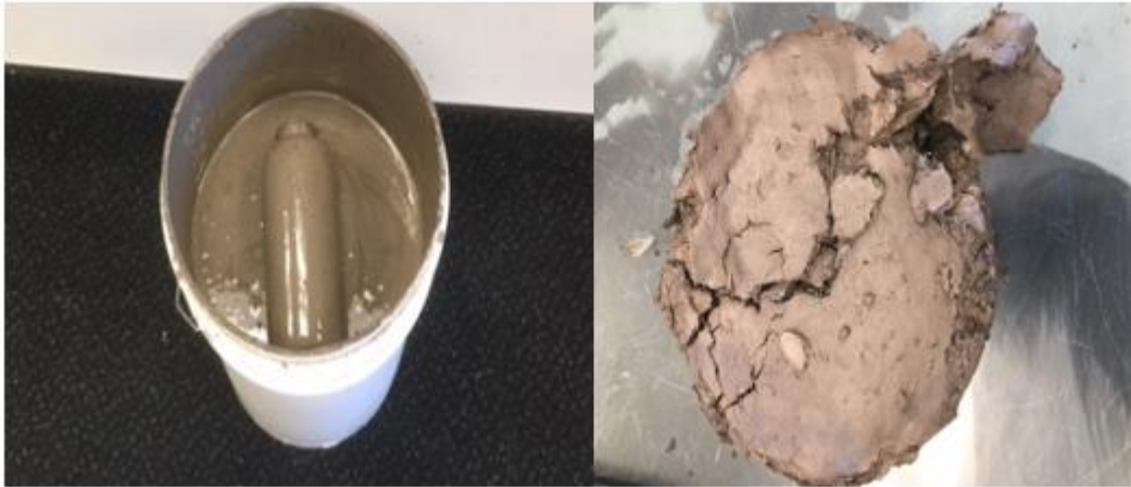
Figure 4.2 A sample of FFT I (left) and a sample of a lime treated FFT cake (right)
