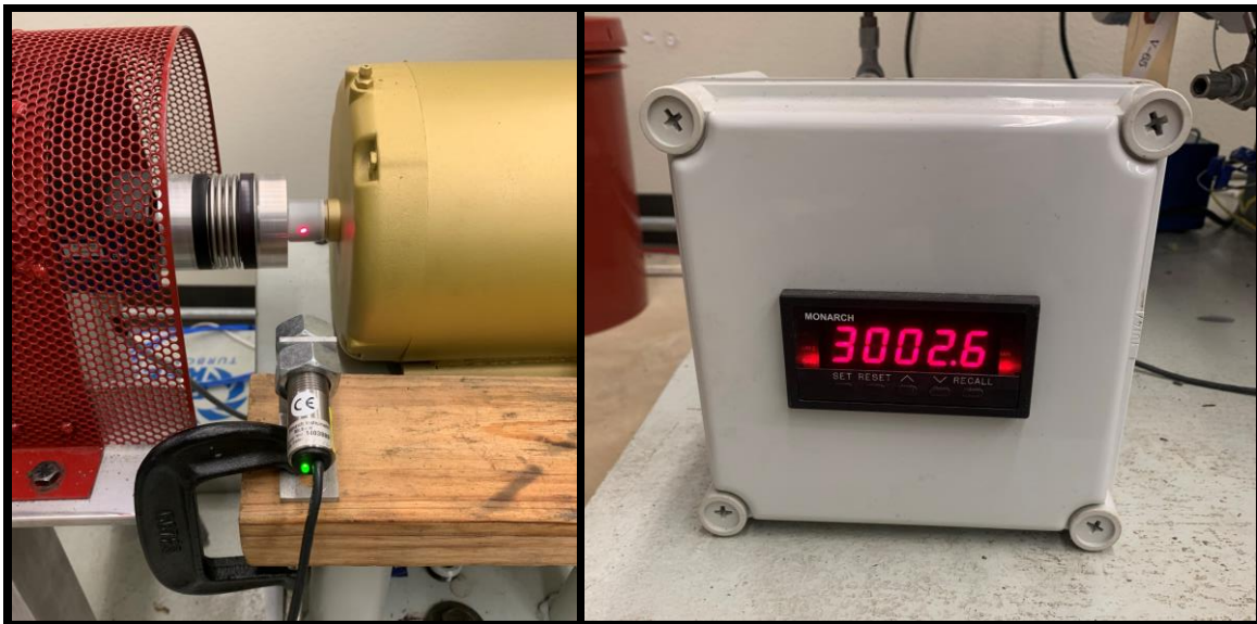
Figure 3.15: Tachometer (left) and its display box (right).
