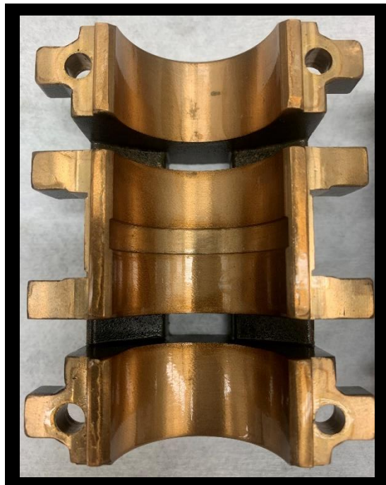
Figure B-93: Motor side top bearing after the unheated, degraded oil, 1000 rpm test.
