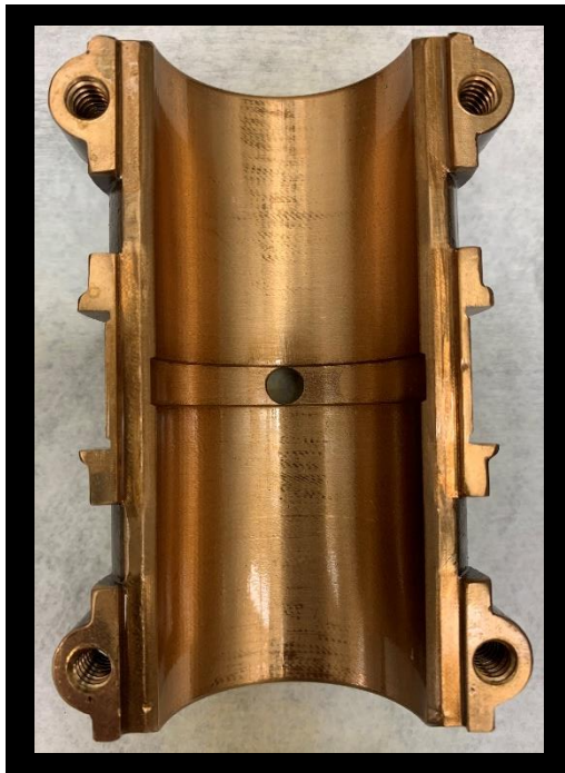
Figure B-122: Motor side bottom bearing after the heated, degraded oil, 1000 rpm test.
