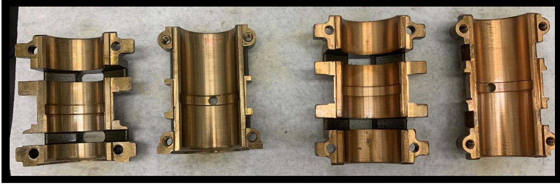
Figure B-131: ZS-1 journal bearings after the heated, degraded oil, 3000 rpm test.
