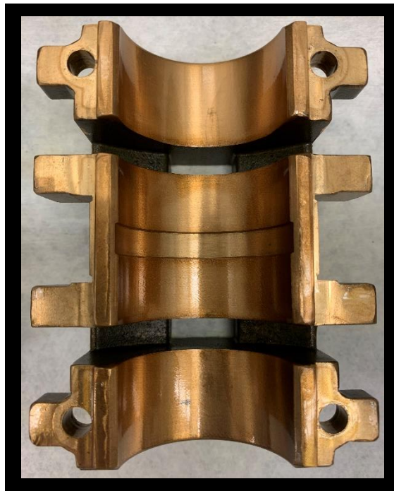
Figure B-121: Motor side top bearing after the heated, degraded oil, 1000 rpm test.
