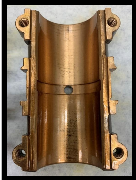
Figure B-81: Motor side top bearing after the heated, fresh oil, 3000 rpm test.
