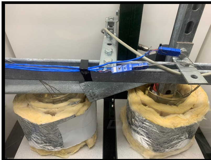
Figure A-5: Top view of the experimental setup for the initial 121°C oil degradation.
