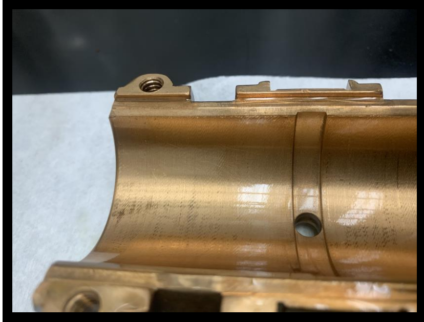
Figure B-109: Shown here is the motor side bottom bearing after the unheated, degraded oil, 3000 rpm test, with slight scoring.
