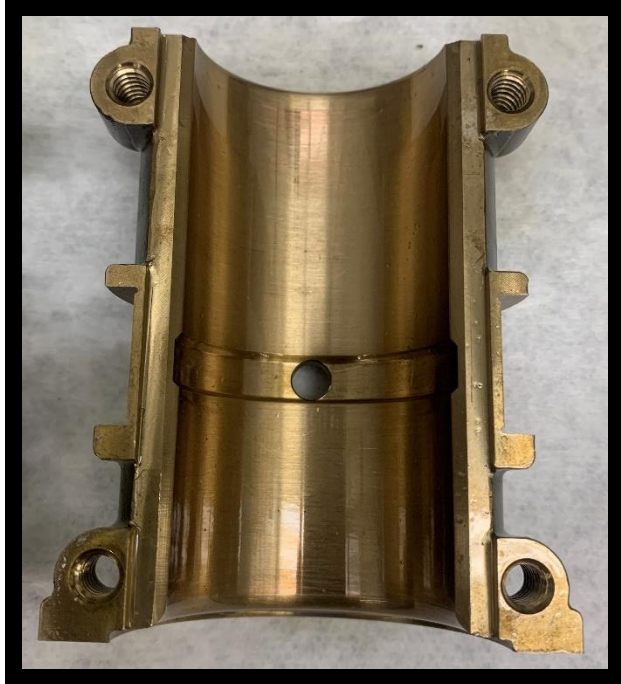
Figure B-53: Governor side bottom bearing after the unheated, fresh oil, 3000 rpm test.
