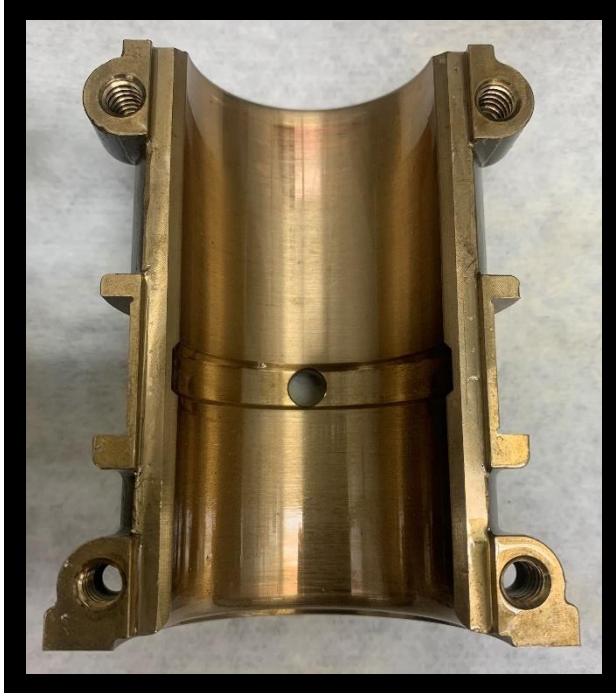
Figure B-105: Governor side bottom bearing after the unheated, degraded oil, 3000 rpm test.
