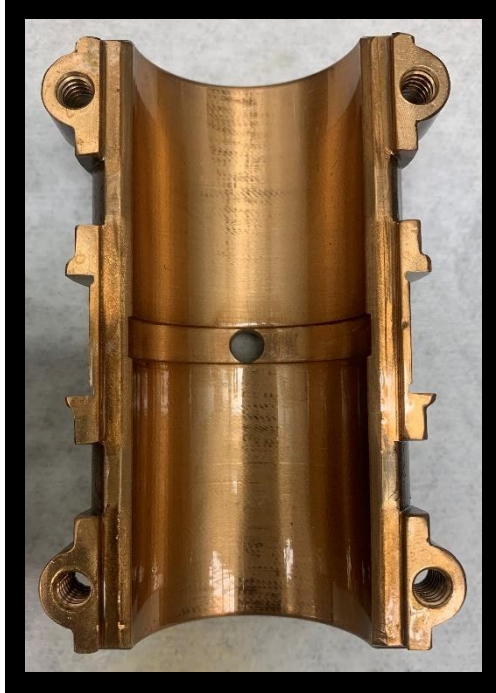
Figure B-107: Motor side bottom bearing after the unheated, degraded oil, 3000 rpm test.
