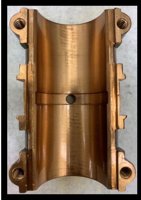
Figure B-135: Motor side bottom bearing after the heated, degraded oil, 3000 rpm test.
