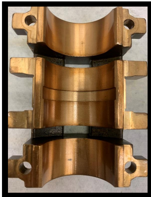
Figure B-134: Motor side top bearing after the heated, degraded oil, 3000 rpm test.
