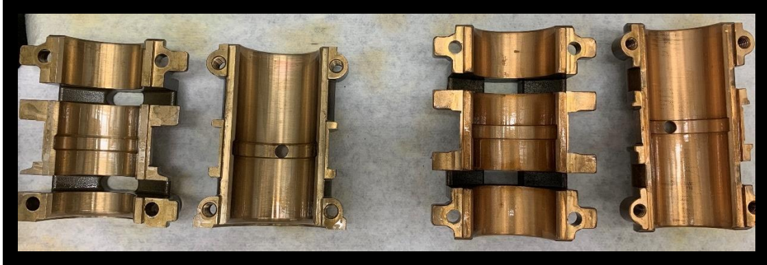
Figure B-77: ZS-1 journal bearings after the heated, fresh oil, 3000 rpm test.
