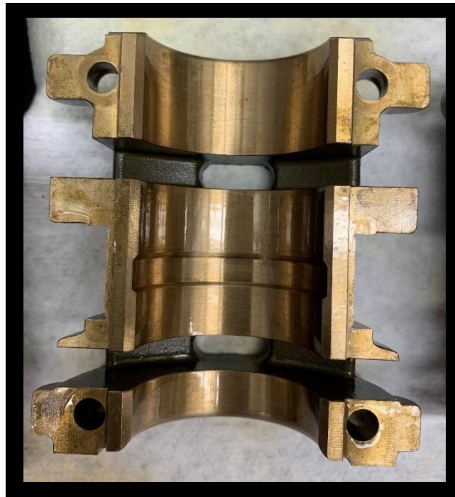
Figure B-78: Governor side top bearing after the heated, fresh oil, 3000 rpm test.
