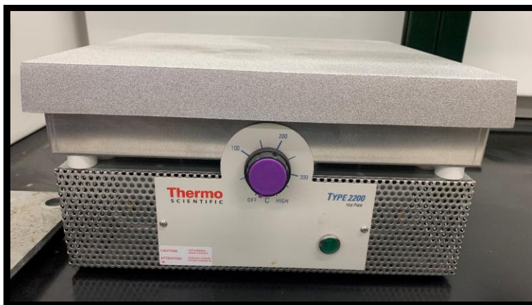
Figure 3.4: Hot plate used for oil degradation tests.
