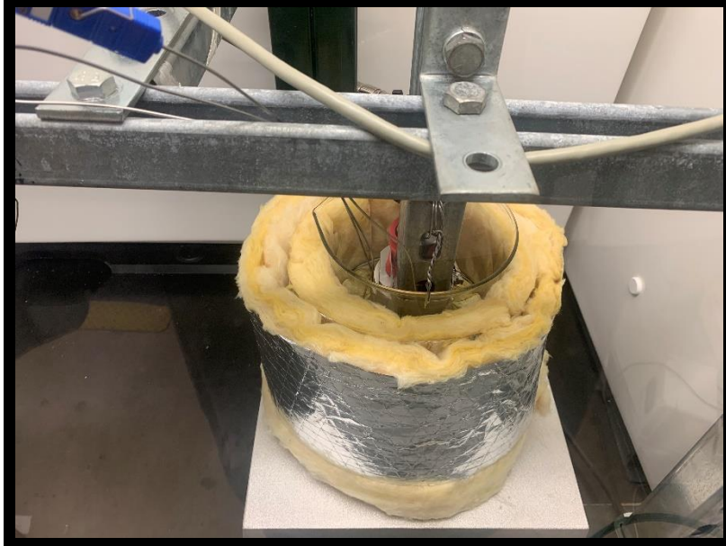
Figure A-11: Oil at the start of the 93°C 10% wet oil degradation.
