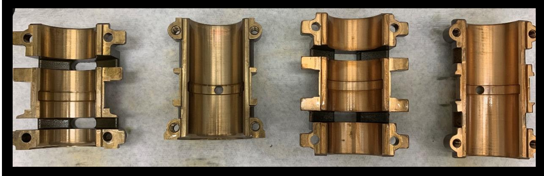
Figure B-118: ZS-1 journal bearings after the heated, degraded oil, 1000 rpm test.
