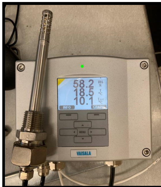
Figure 3.14: Front display and measurement probe of the hygrometer.
