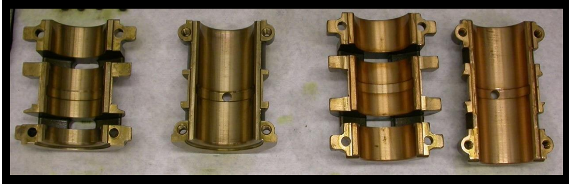
Figure B-64: ZS-1 journal bearings after the heated, fresh oil, 1000 rpm test.
