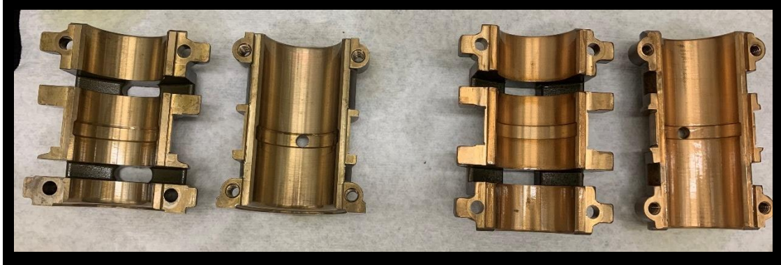
Figure B-51: ZS-1 journal bearings after the unheated, fresh oil, 3000 rpm test.
