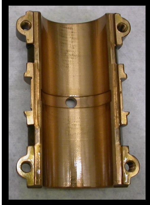
Figure B-68: Shown here is the motor side bottom bearing after the heated, fresh oil, 1000 rpm test.
