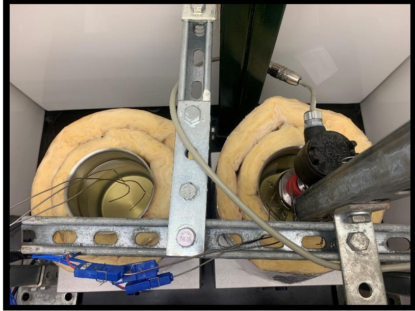
Figure A-23: Oil at the start of the second 121°C oil degradation.
