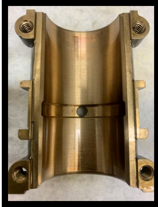
Figure B-133: Governor side bottom bearing after the heated, degraded oil, 3000 rpm test.
