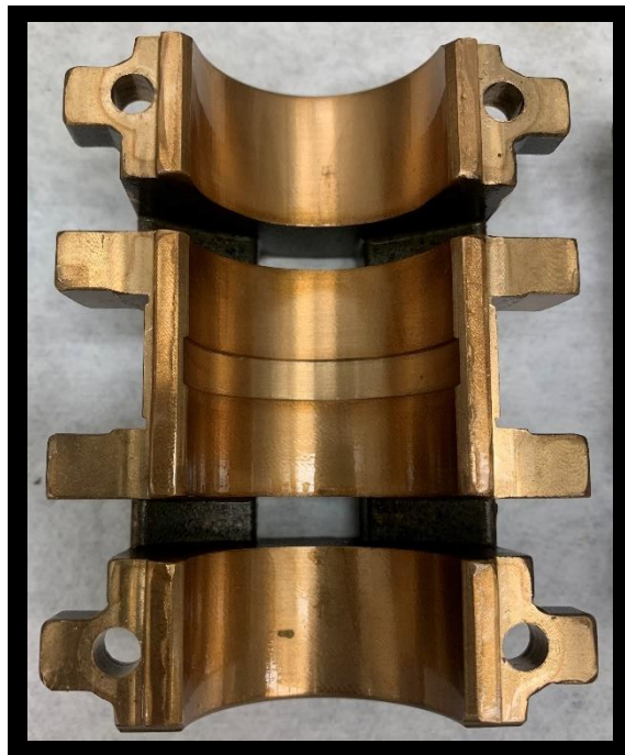
Figure B-54: Motor side top bearing after the unheated, fresh oil, 3000 rpm test.
