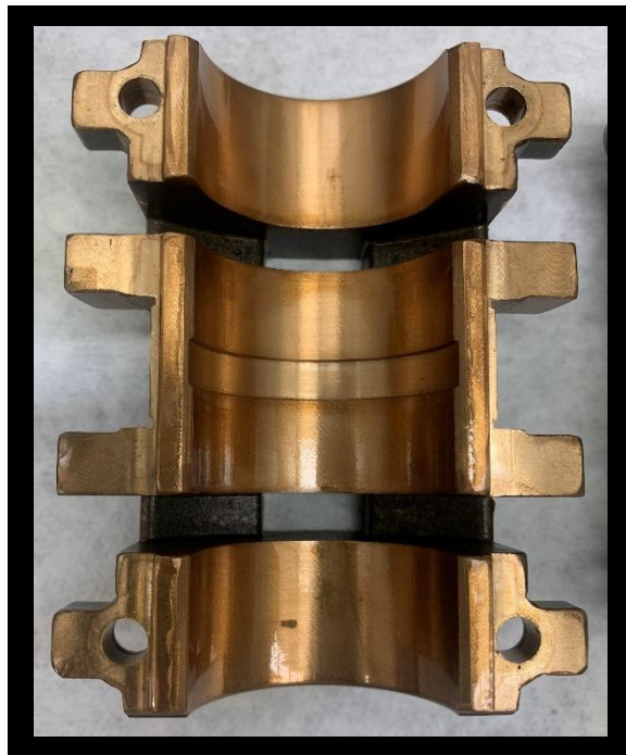
Figure B-106: Motor side top bearing after the unheated, degraded oil, 3000 rpm test.
