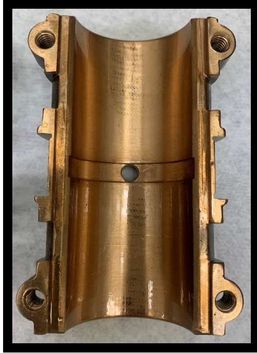
Figure B-55: Motor side bottom bearing after the unheated, fresh oil, 3000 rpm test.
