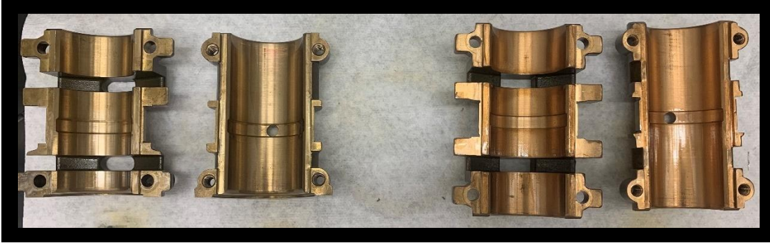
Figure B-103: ZS-1 journal bearings after the unheated, degraded oil, 3000 rpm test.
