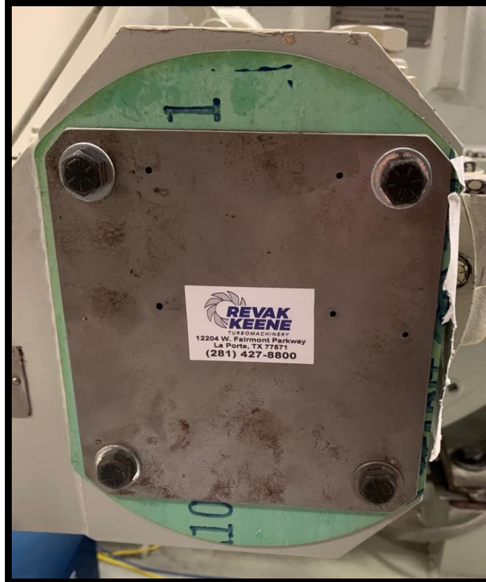
Figure 3.21: Steel plate used to seal the governor penetration.
