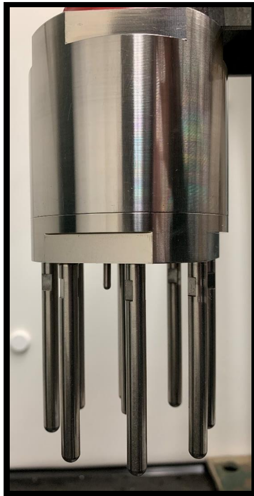
Figure 3.6: Viscometer used for oil degradation tests.
