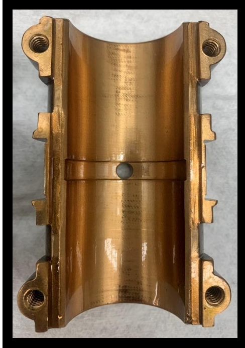
Figure B-94: Motor side bottom bearing after the unheated, degraded oil, 1000 rpm test.
