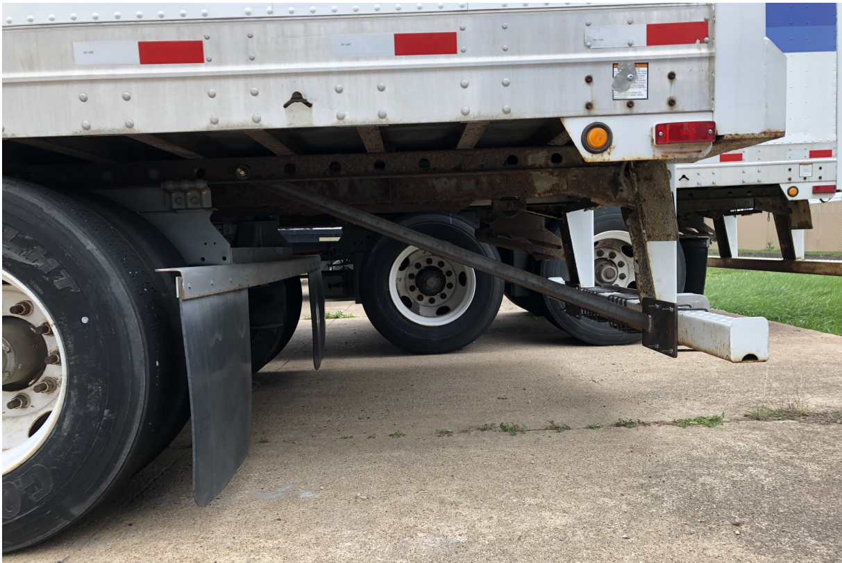
Figure 5.3: Welded Steel Supports Reinforcing the Bumper of the Leading Trailer
