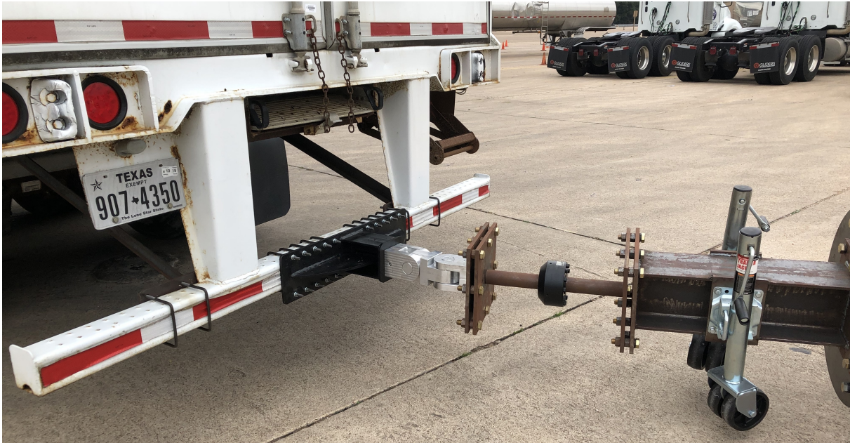
Figure 5.4: Double Pin Joint Bolted to Leading Trailer
