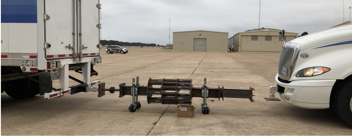
Figure 5.2: Prototype Tow Bar during Assembly
