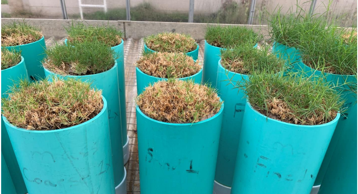
Figure 3.23: A closer view of the 2019 lysimeters after the dry-down study and recovery phase with the following treatments from left to right: Coarse SCG Mass, Sand, Fine SCG Mass.
