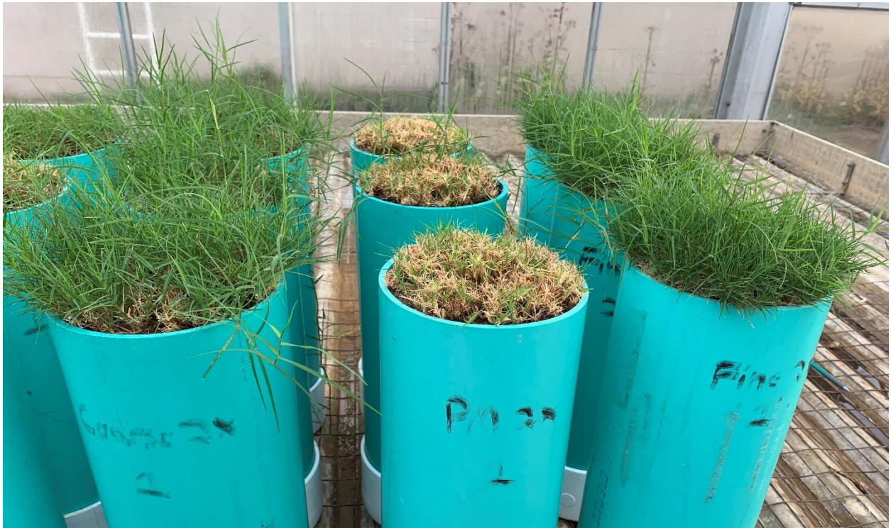
Figure 3.24: A closer view of the 2019 lysimeters after the dry-down study and recovery phase with the following treatments from left to right: Coarse SCG 20%, Peat Moss 20%, Fine SCG 20%.
