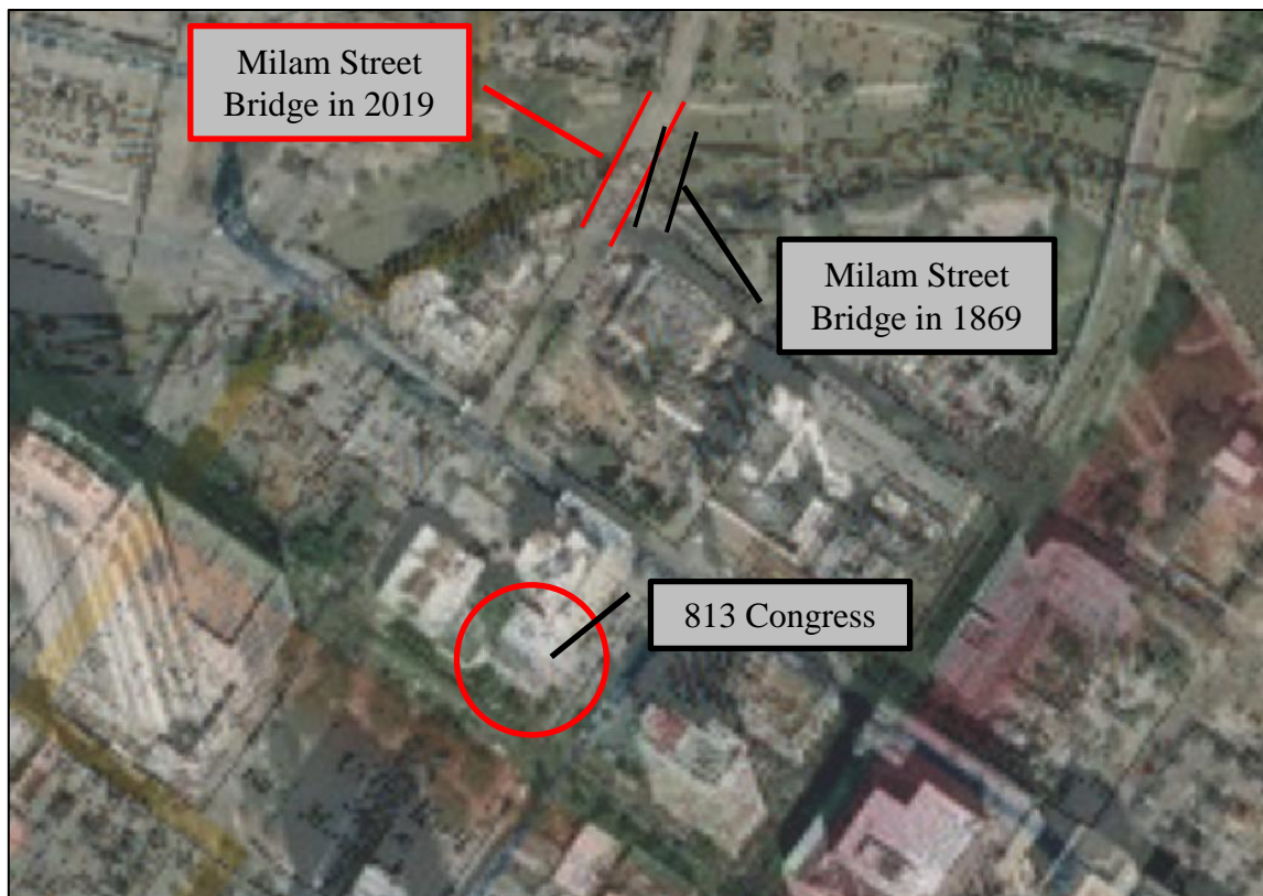
Figure 25 The 1869 Wood Map of Houston (Wood, 1869) georeferenced to 2019 satellite imagery (Bing Maps, 2019) of the Houston downtown near the Milam Street Bridge. The 1869 is set to 50 percent opacity. Courtesy the author.
