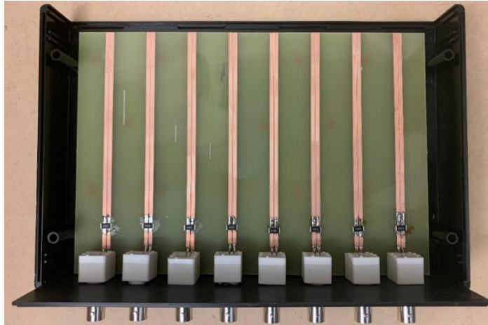
Figure II-6. 16-channel mock preamplifier box. Eight of the 16 channels of the mock preamp box are shown including the transmission lines, 0.5\Omega resistors in shunt, and BNC panel-mount connectors.
