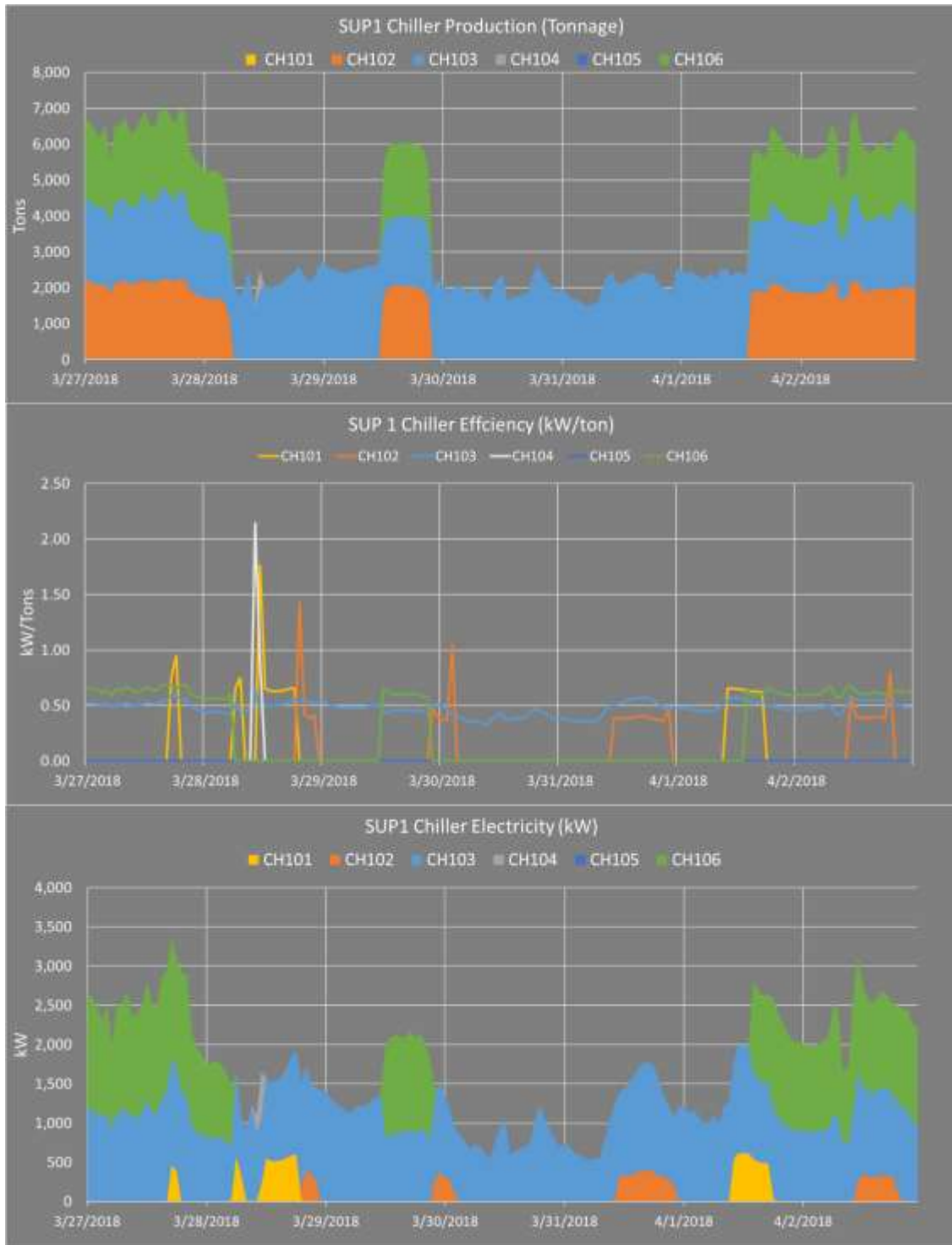
Figure III.1. Chiller performance plots.
