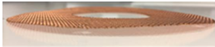
Figure 28. Photograph of a single layer of 20 OPI mesh depicting the inherent waviness in the thin structure.
