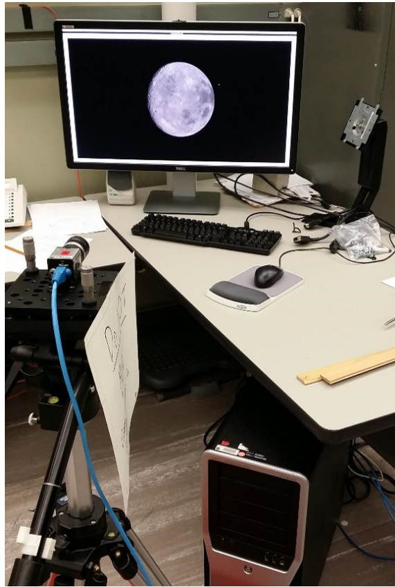
Figure IV.7: Preliminary camera calibration for capture of synthetic EDGE images in the Electro-Optics Lab at JSC. An EDGE rendering of the Moon is being displayed on a 4k display while a tripod mounted camera captures live footage.
