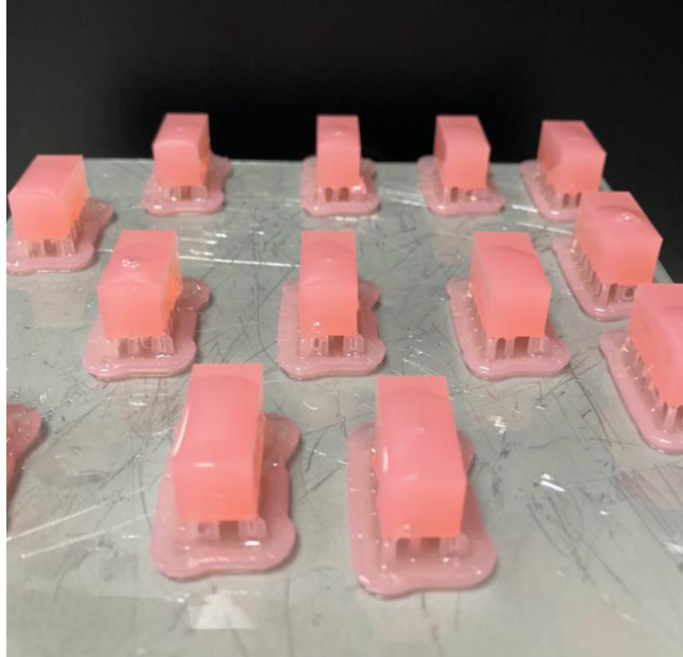
Figure 3. 3D printed denture base specimens prior to post-processing
