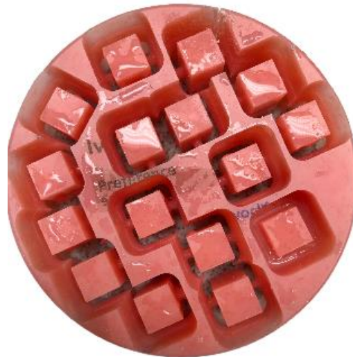
Figure 5. IvoBase CAD PMMA disc following subtractive manufacturing (10 mm x 10 mm x 20 mm)
