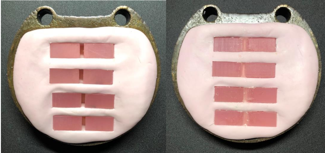
Figure 8. Fabrication of experimental specimens with denture liner. Image on left illustrates 3 mm of space provided for reline material between two denture base samples each measuring 20 mm in length. Image on right shows reline material bonded to both denture base samples prior to removal from rubber silicone investment.
