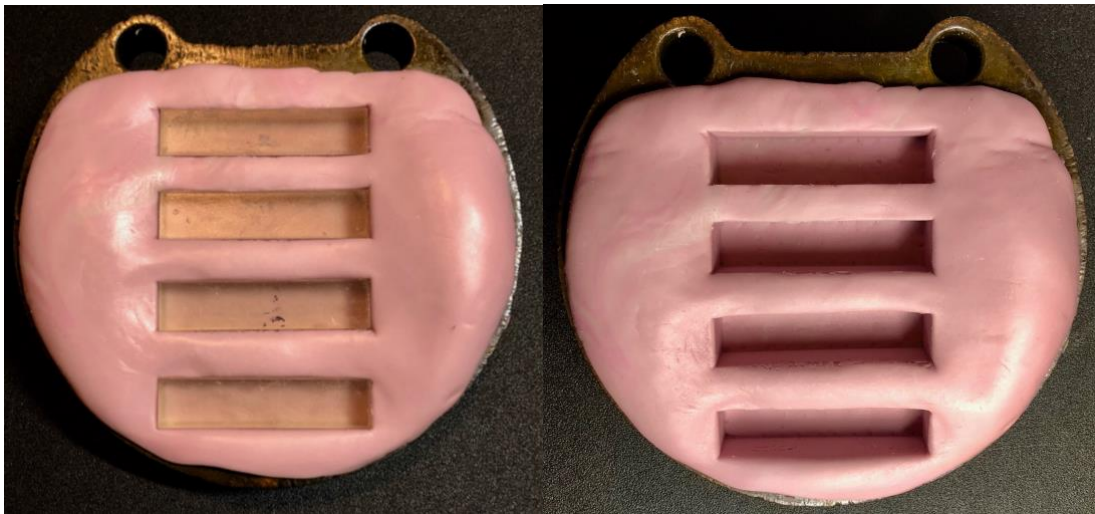
Figure 7. Template molds. Photo on left illustrates investment of the 3D printed template bars (10 mm x 10 mm x 43 mm). Addition of 3 mm was included to allow for 3 mm of space for reline material. Image on right illustrates spaces for denture base specimens after removal of 3D printed bars once rubber silicone had set.
