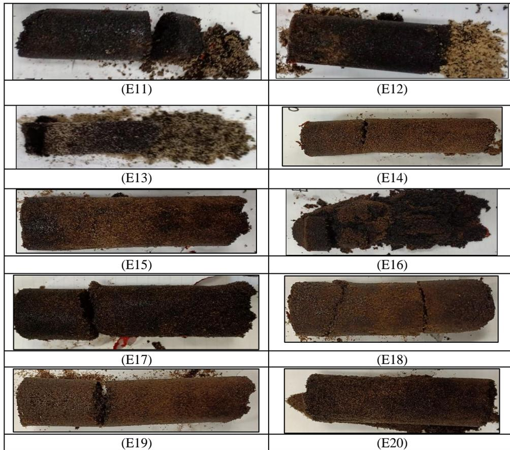
**Figure 4.20—Spent rock images for all experiments conducted with Oil 2. Injection is from left (inlet) to right (outlet). For experiment naming, refer to Table 3.2.**
