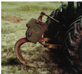
Single-shank ripper mounted on a 40-hp tractor.
