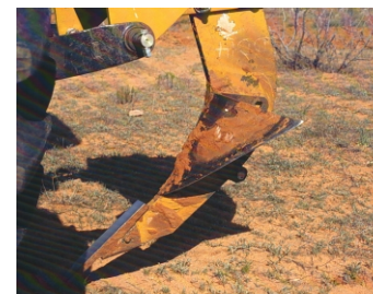
Furrow opener for contour furrowing or wing ripping.
