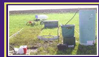
Photograph 2. Equipment used for the study including the nurse-tank, pump, applicator, runoff plot, sampling station, data logger and capture tank.
