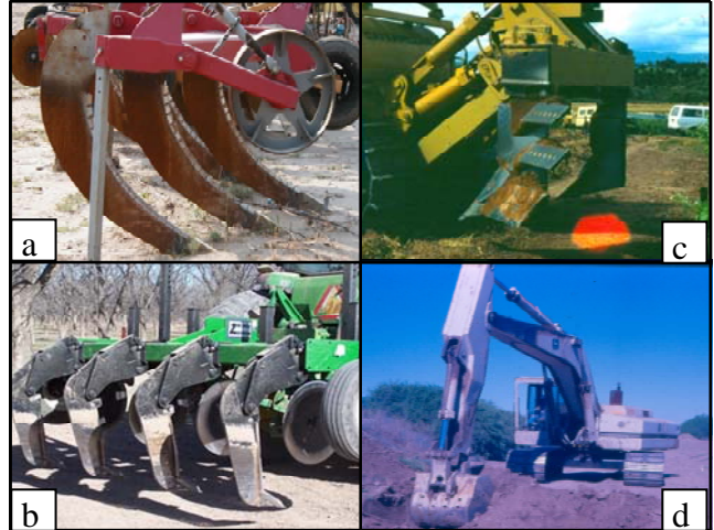
Fig. 3. Ripper shank, subsoiling shank, deep chisels, and an excavator used by growers in the El Paso Valley
