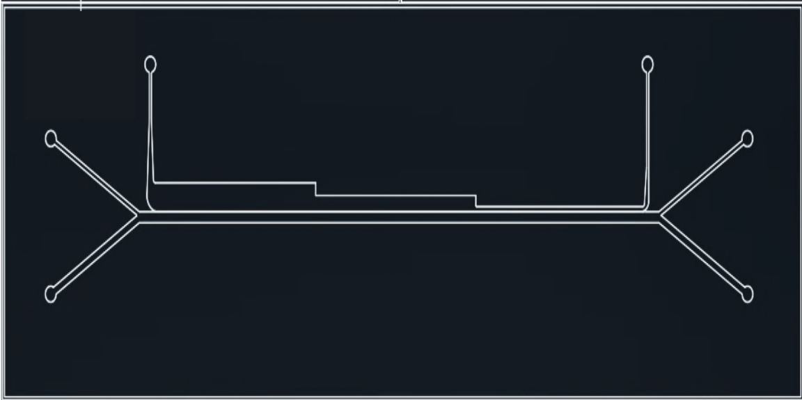
Figure A. 6-2 Mask design for acoustic microfluidic channel with staircase echo-channel.
