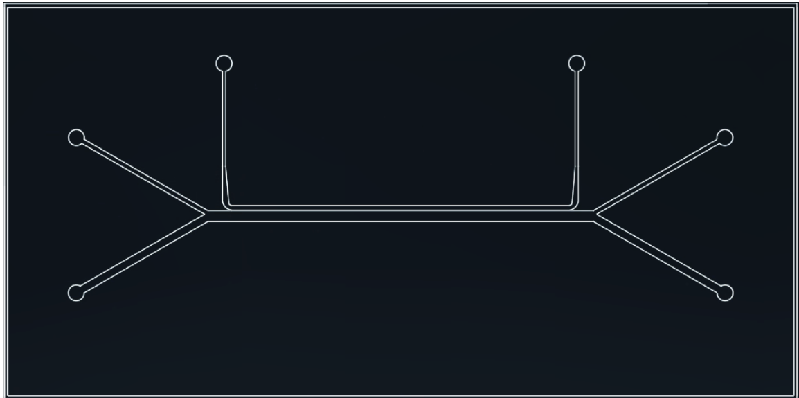
Figure A. 6-1 Mask design for acoustic microfluidic channel with straight echo-channel.
