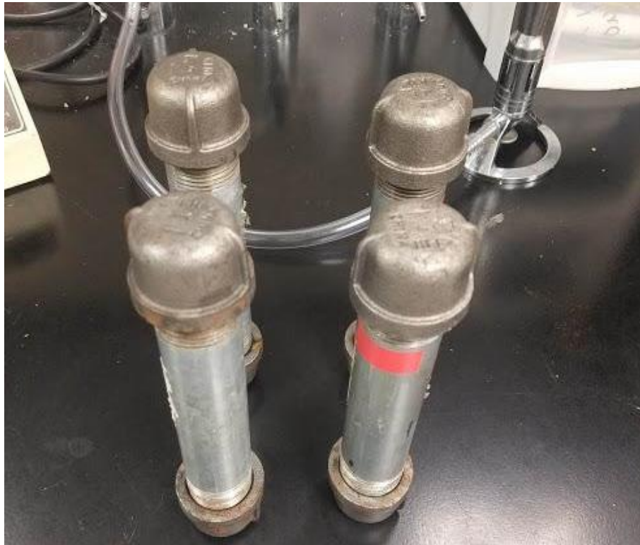
Figure 1. Metal vessels used to hold sample materials during thermal rendering experiments of chicken feathers or chicken blood.
