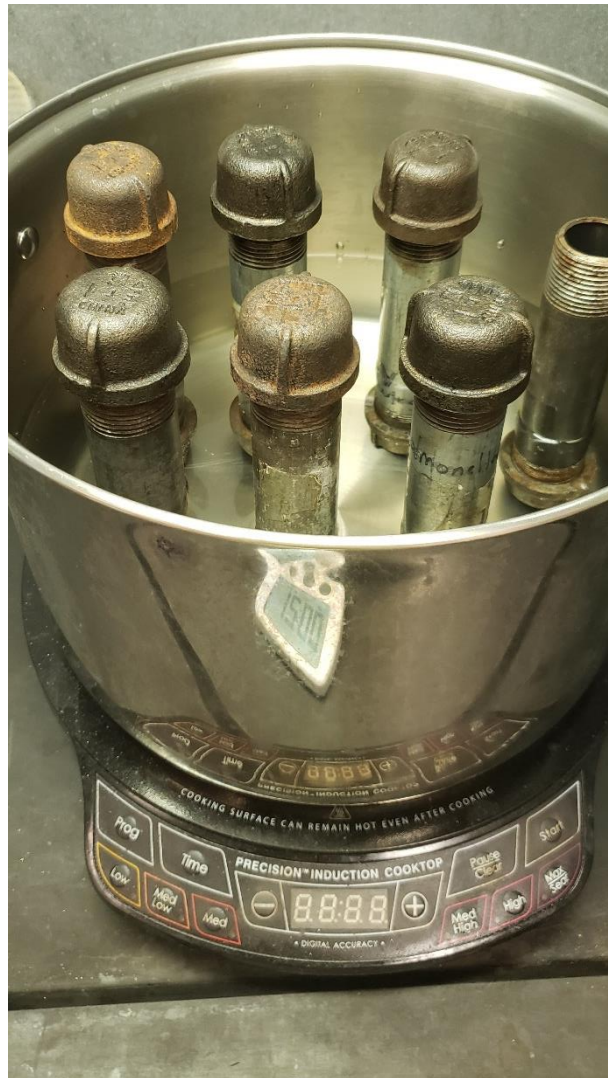
Figure 2. Metal vessels immersed in distilled water in a stainless-steel cookpot on a Precision™ induction cooktop.
