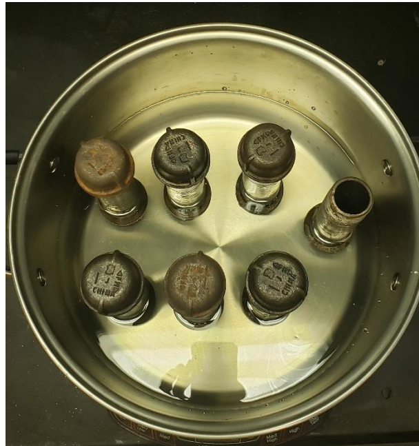
Figure 3. Metal vessels spaced sufficiently in order for sample separation.
