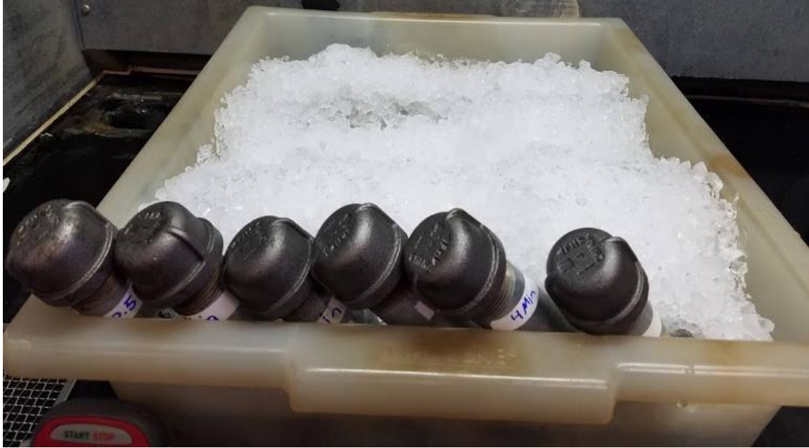
Figure 4. Metal vessels in ice-laden cold water (0°C) to halt heat transfer.
