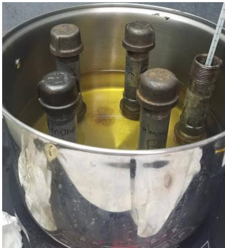
Figure 5. Metal vessels immersed in peanut oil in a stainless-steel cooktop on a Precision™ induction cooktop.
