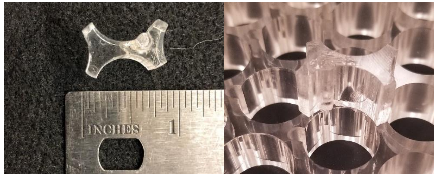
Figure 4.3 Interior Blockage and spacer plate to offer a visual of how the blockage will interface with rods.
