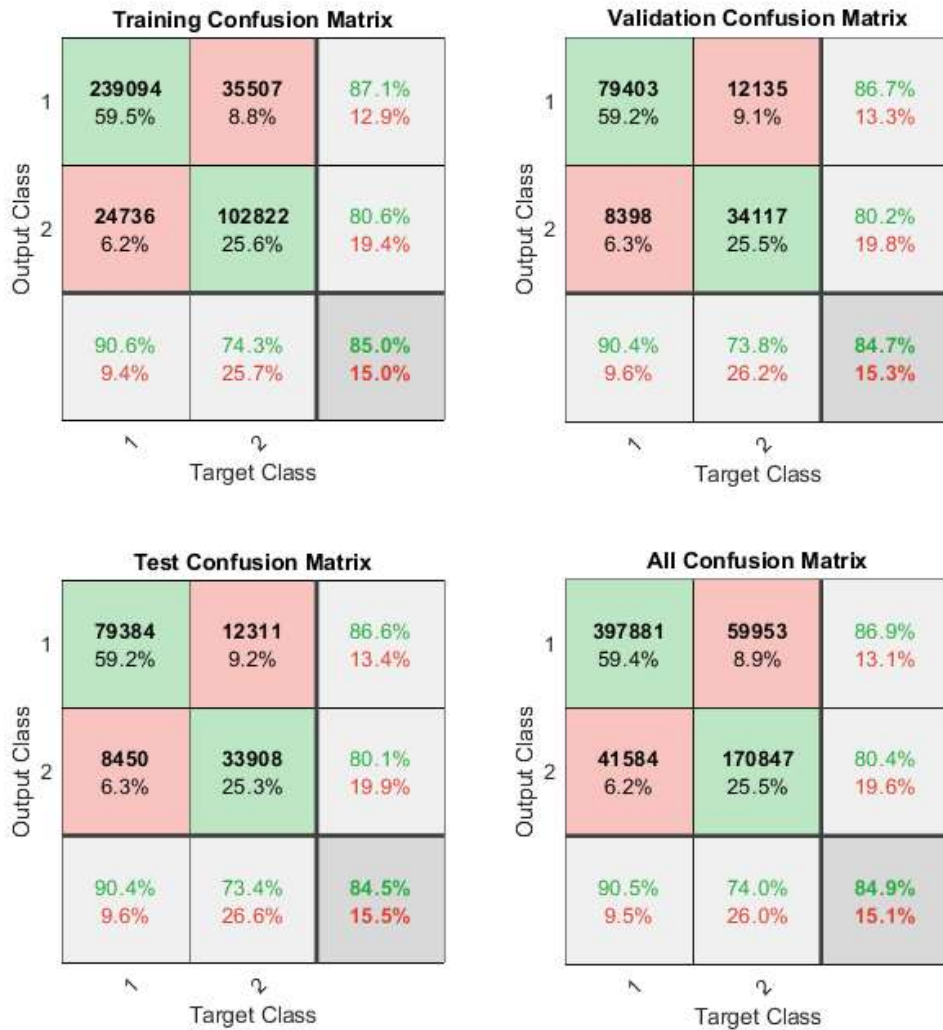
Figure 5.9 Confusion Matrices for Network with Three Hidden Layers with 1000, 1000 and 100 Neurons with Augmented Data.
