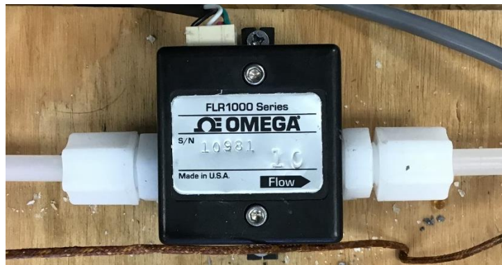
Figure 12 Omega Flow Meter FLR 1010 used to measure the flow rate of HTF
