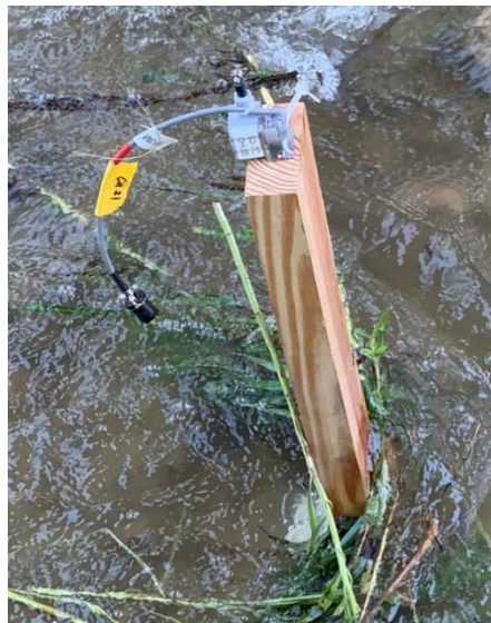
(c) Example of an Installed String Potentiometer
