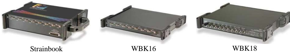
(a) Main Data Acquisition Box and Extension Modules (Reprinted from Measurement Computing 2014 )
