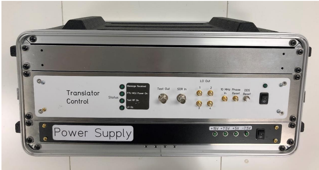
Figure 4.3: Control unit, containing, from top to bottom, empty slot for transmit translation unit, translator control unit, and power supply unit.
