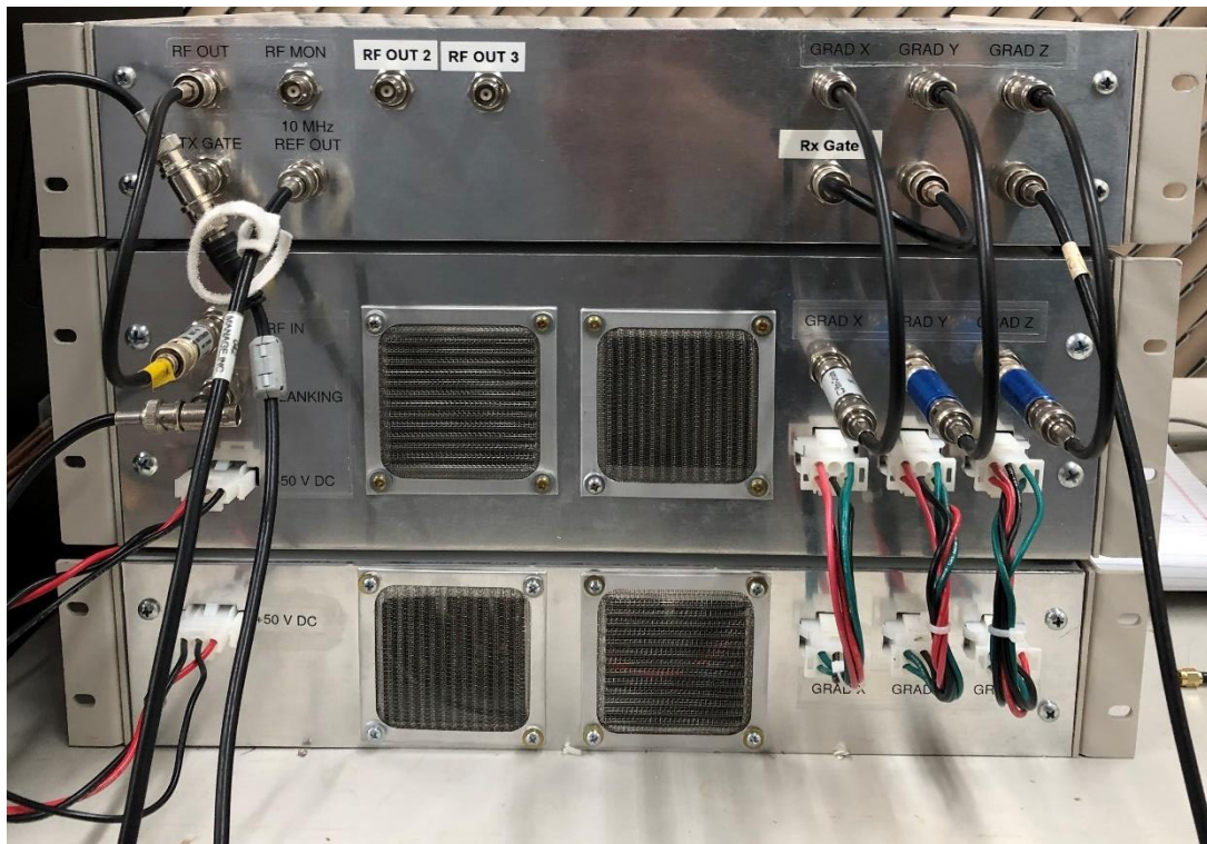
Figure 5.2: Front of full broadband system. Units are, from top to bottom, small signal unit, power amplifier unit, and power supply unit.
