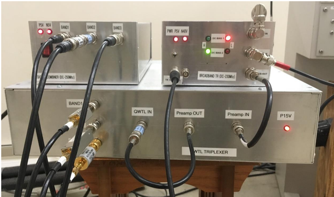
Figure 5.10: Triplexing front-end and broadband T/R switch. Top units are, from left-to-right, the broadband signal combiner and the broadband T/R switch. The bottom unit is the signal triplexer and preamplifier unit.
