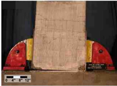
Figure 1.11. Non-emulative rocking column connection with friction links (Reprinted from Morgen and Kurama 2004).
