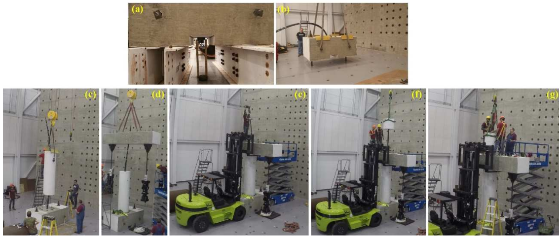
Figure 7.29. Test setup assembly steps for RC rocking specimen: (a) foundation blocked to pass the strands; (b) lowering the foundation block; (c) lowering segment(s); (d) lowering cap-beam-actuators assembly; (e) placing load cells in position; (f) lowering PT anchorage block; (g) post-tensioning.
