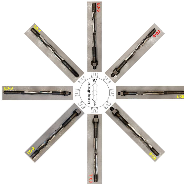
Figure 7.73. PUED-2 specimen: extracted view of ED links.
