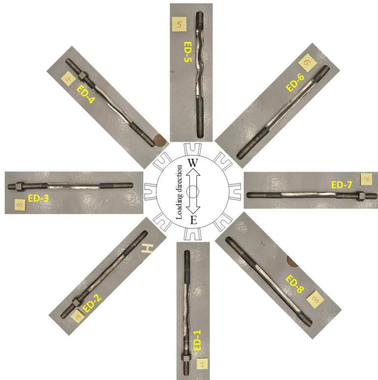
Figure 7.57. PUED-1 specimen: extracted view of ED links.
