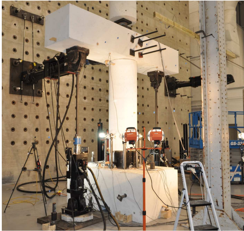
Figure 7.15. PUEd column test setup.
