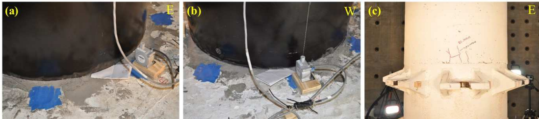
Figure 7.95. PU column at 1.8×DE (1.2×MCE) at the loading rate of 1.08 in/sec: (a) and (b): gap size increased on east and west sides; (c) crack in cover concrete.
