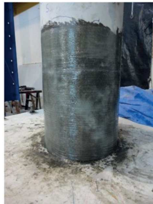
Figure 1.8. Posttensioned non-emulative column-footing connections with FRP wrap (Reprinted from White and Palermo 2016).
