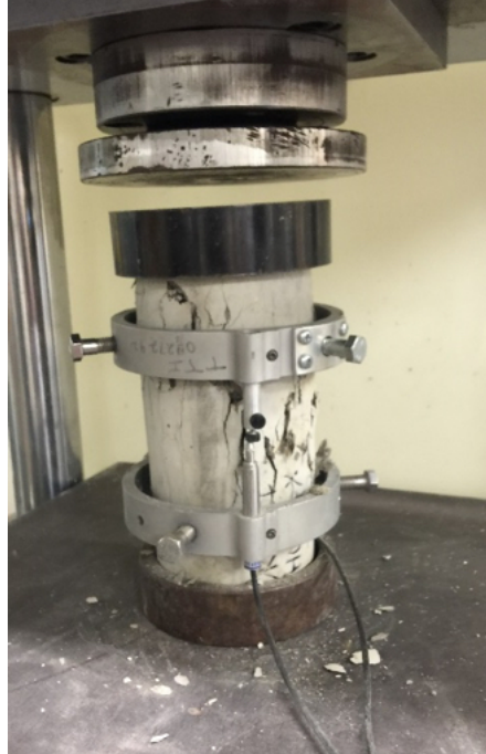
Figure 5.1: Experimental set-up for uni-axial compression test for RAP-PCC cylindrical specimens [1]
