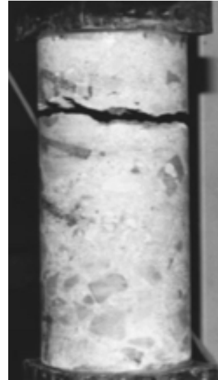
(b) Crack pattern observed experimentally under uni-axial tensile loading in the vertical direction [63]
