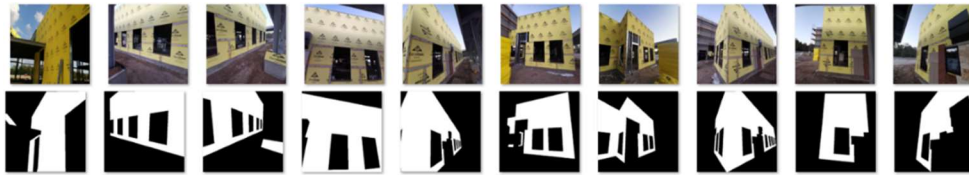
Figure 4 Training images and corresponding labeled images for detecting sheathing plywood
