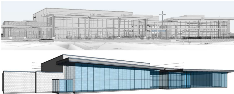
Figure 2 A rendering of the church and corresponding BIM model
