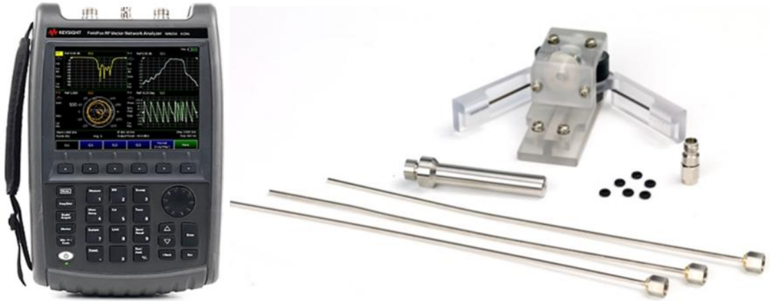
Figure 2.1 - Both the vector network analyzer and dielectric probe kit utilized to measure the complex permittivity of the sample
