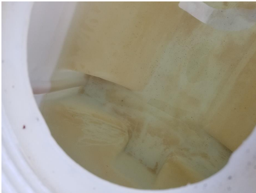
Figure 6.3. Final cleaning run resulting in clear water indicating clean internals.
