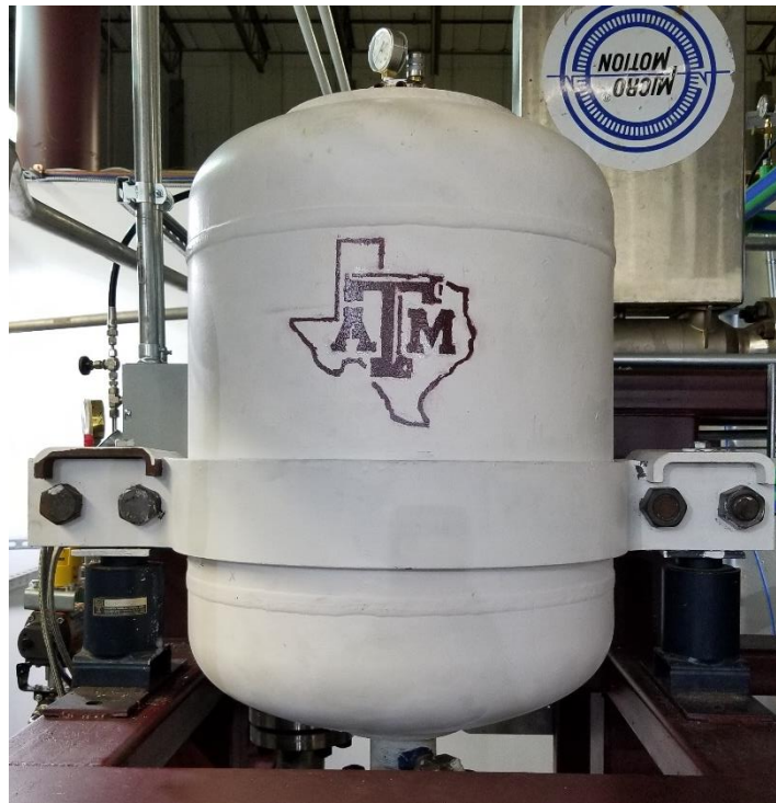
Figure 2.10. Surge suppressor tank with Nitrogen-filled bladder to pressurize the process fluid in the CHF facility.
