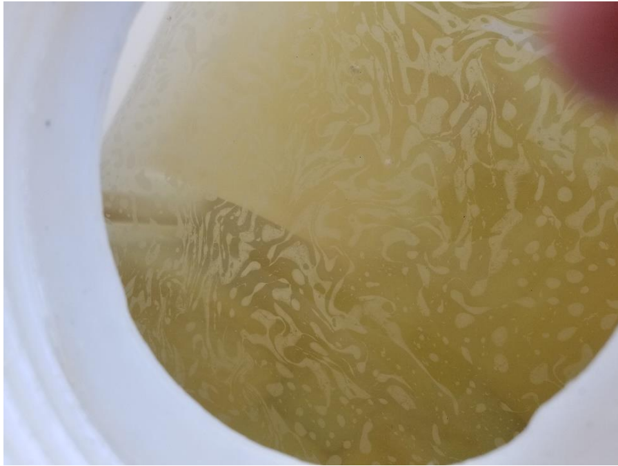
Figure 6.2. Second facility cleaning run which yielded remaining rust particles and cleaning product.
