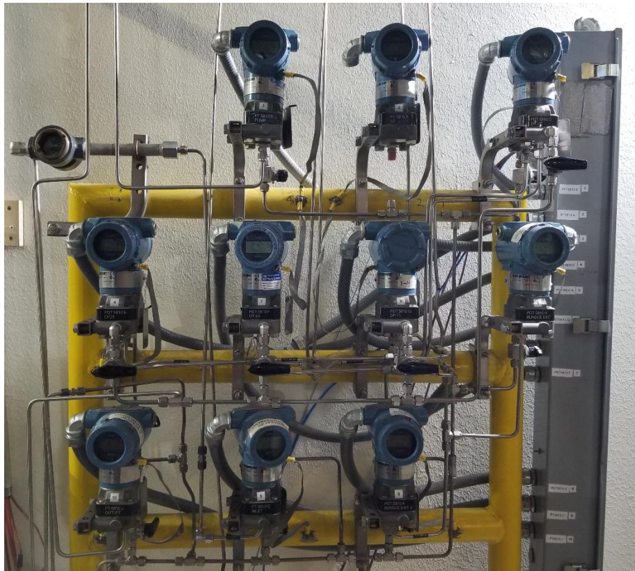
Figure 3.5. Pressure transducer grid – differential and gauge – connected to various points along the CHF facility.
