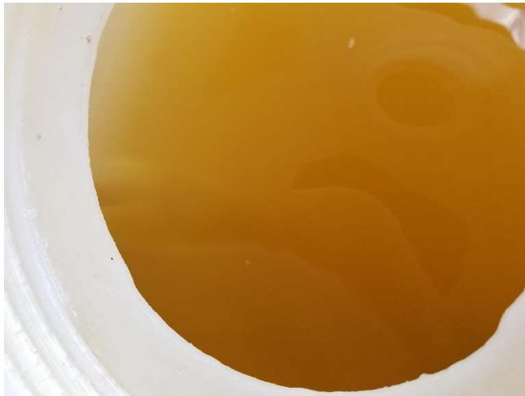
Figure 6.1. First run facility drain water with suspended rust from facility internals.
