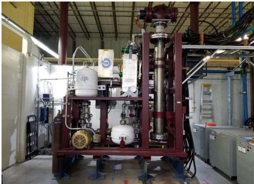
Figure 2.1. TAMU CHF test facility with all components installed.
