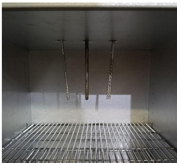
Figure 3.3. Closest approachable positioning distance between the reference probe (center) and the uncalibrated temperature sensors.
