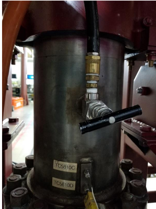
Figure 5.1. Valve A connected to the test section which is used to fill the system.
