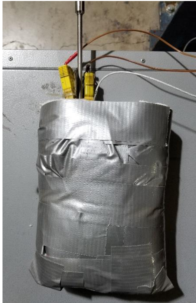
Figure 3.4. Ceramic insulation pouch used to collect steady-state room temperature data.
