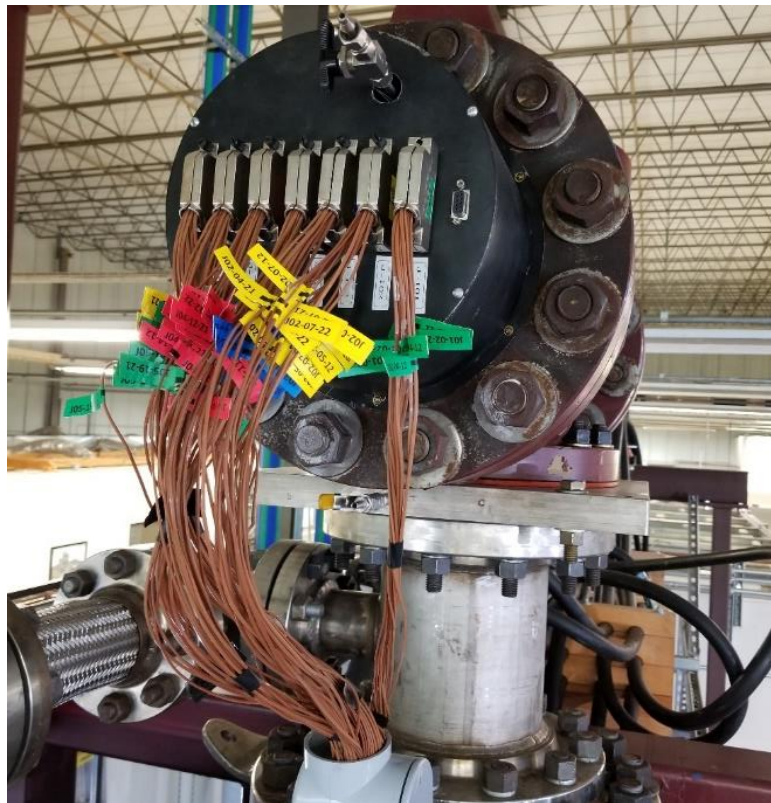
Figure 3.1. Axial rod thermocouples routed to the DAQ from the test section.
