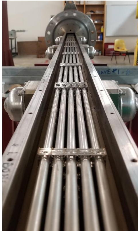
Figure 2.6. Rod bundle in flow duct, with spacer grids and mixing vanes.
