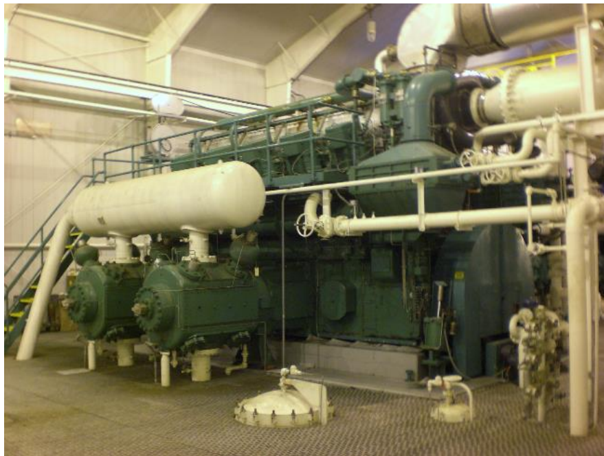
Figure 15: Cooper-Bessemer GMWH-10C used for data collection.
