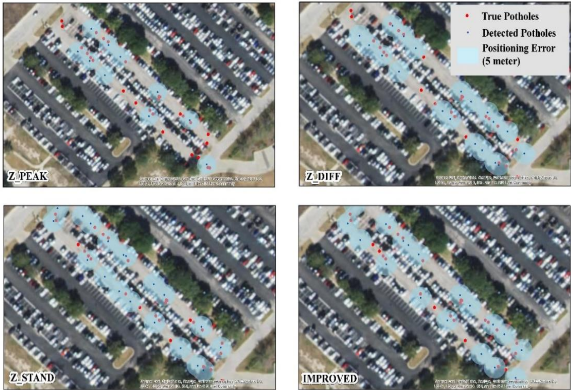
Figure 3.9 True pothole distribution and four pothole detection methods' results from 5 laps (red dot: true pothole; blue dot: detected pothole; light blue buffer: positioning error tolerance).
