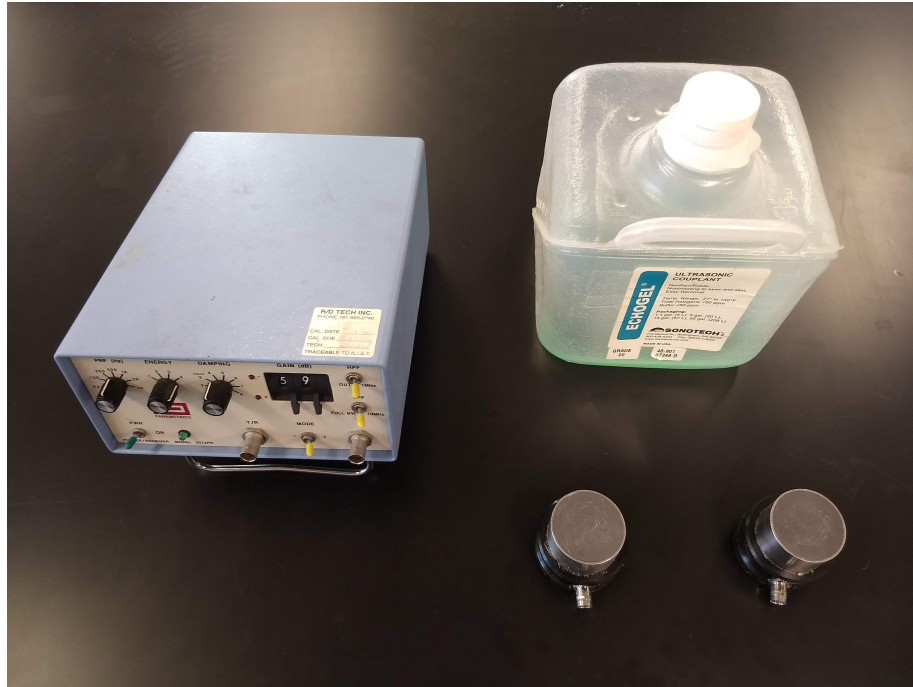
Figure 2.5: Ultrasonic Transducers (right bottom), Coupling Agent (right top), and Ultrasonic Pulse Receiver (left)
