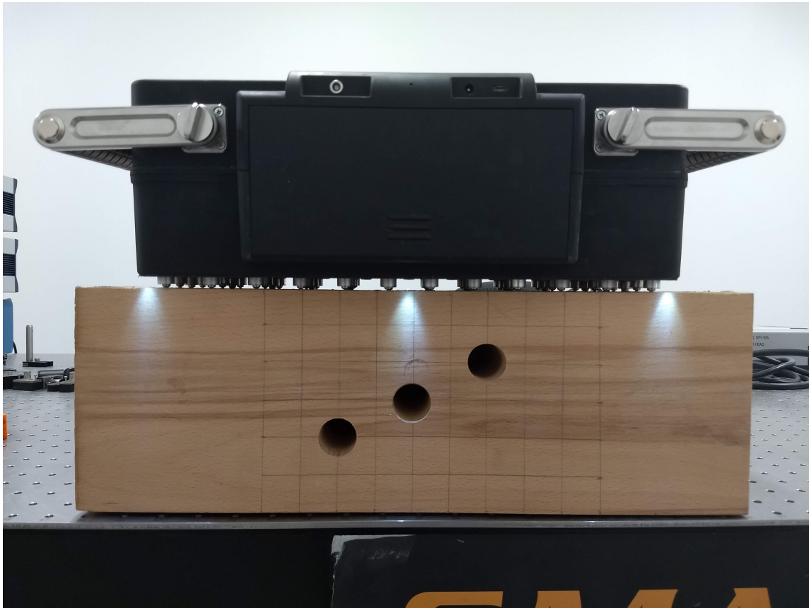
Figure 6.14: Wood Specimen with Three \varnothing 25.4 mm Damage at Different Depth
