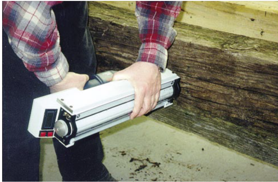
Figure 2.1: Resistance Drill in Use Reprinted from Brashaw et al. (2005)
