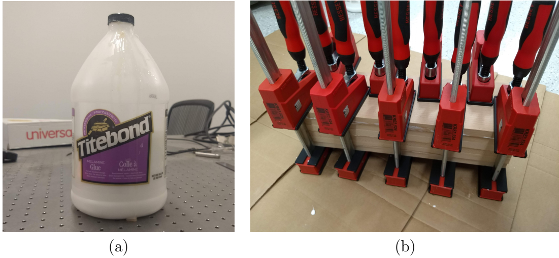
Figure 6.2: Construction of Wood Specimen: (a) Melamine Wood Glue for Wood Specimen and (b) Clamping Wood Specimen
