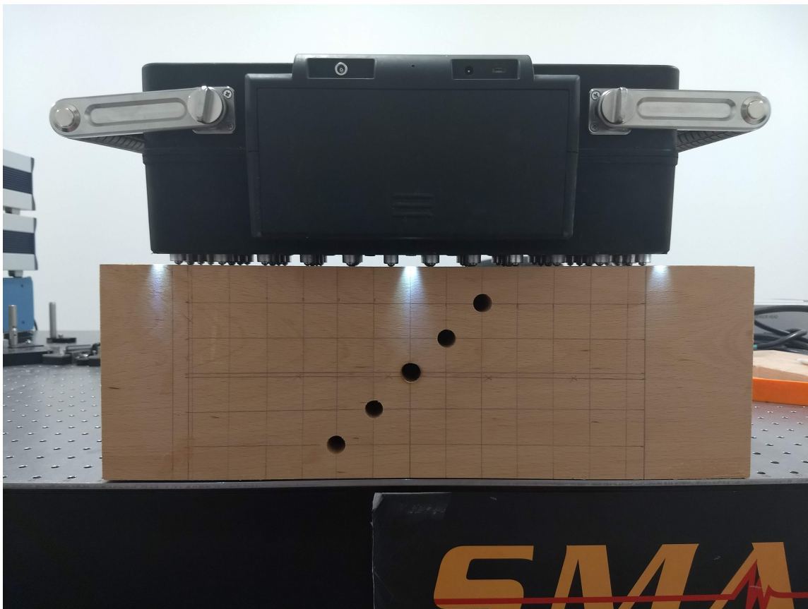
Figure 6.8: Wood Specimen with Five \varnothing 12.7 mm Damage at Different Depth
