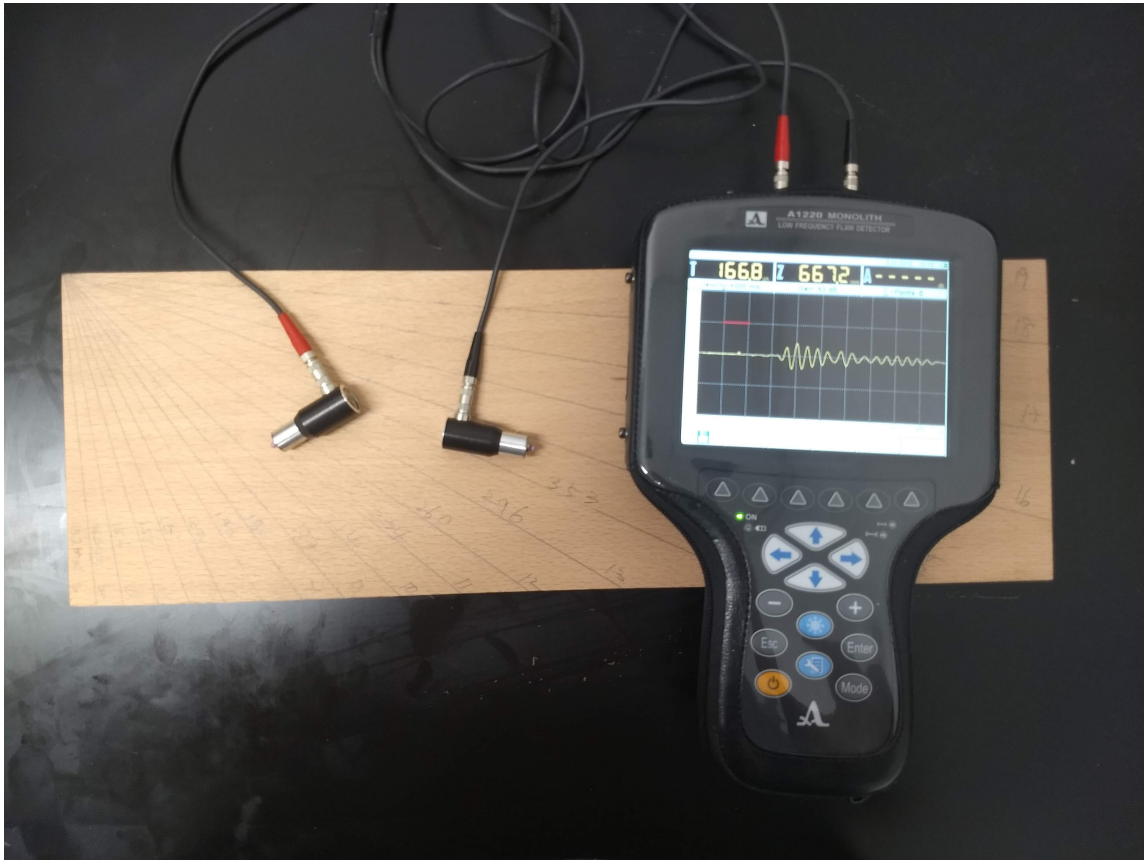
Figure 6.4: Low-Frequency Ultrasonic Flaw Detector A1220 Monolith (Electronic Equipment) and Drypoint Contact Shear Wave Transducer S1802 (Probe)
