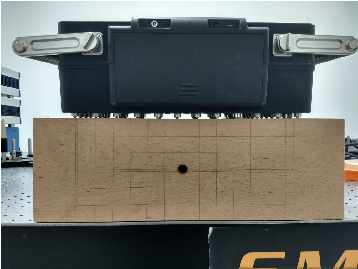
Figure 6.5: Wood Specimen with One \varnothing 12.7 mm Damage at Center
