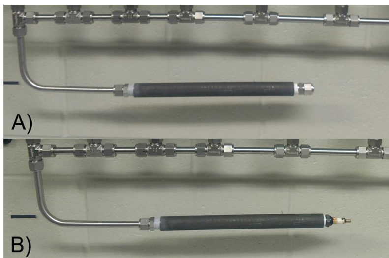
Figure 8. Ignition spark plug tester on the manifold. A) Shows the tester in its normal configuration with a plug at the end. B) Shows the tester being used to test the ignition spark plug.
