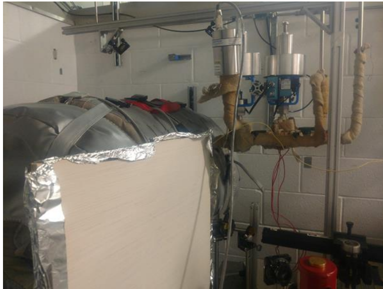
Figure 35. Heat shield between the heated vessel and the J10D Series Indium Antimonide detector. Also visible are the HeNe laser tube and a couple of the mirrors used to pass the laser beam through the vessel.
