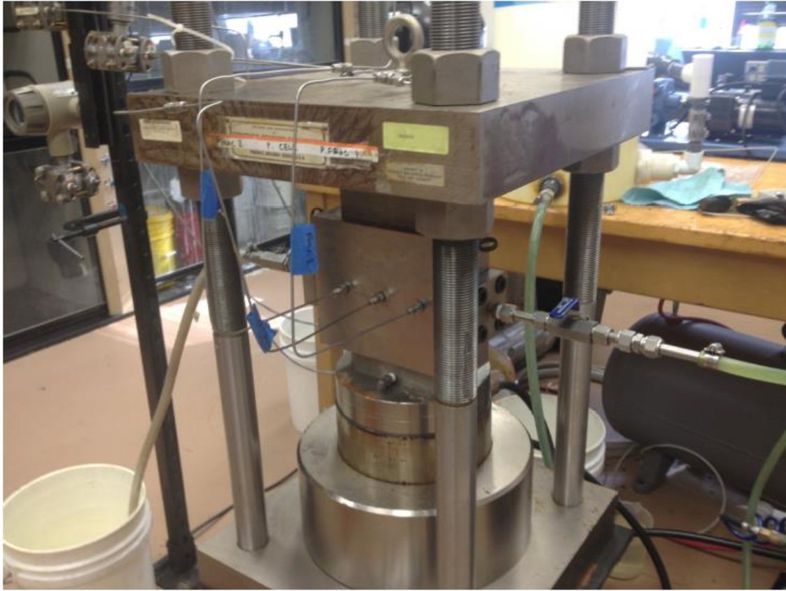
Figure 16 Acid fracture conductivity cell in the middle of loading frame of acid fracture conductivity measurement apparatus (Reprinted from Underwood 2013)
