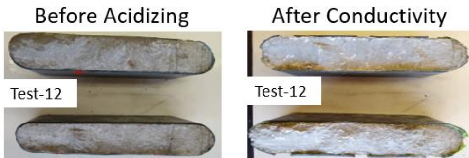
Figure 28 Surface characterization of test-12 – Pore-filled distribution
