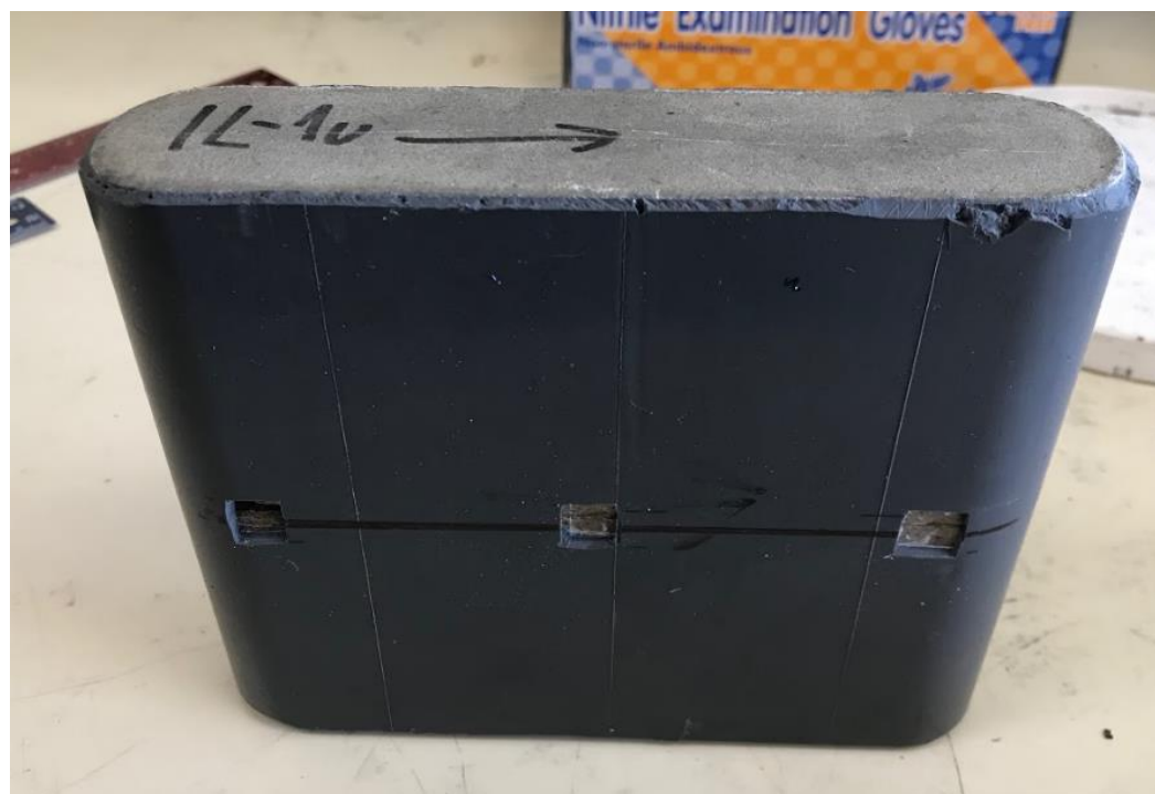
Figure 11 Rock sample preparation for acid fracture conductivity measurement (Reprinted from Jin 2019)
