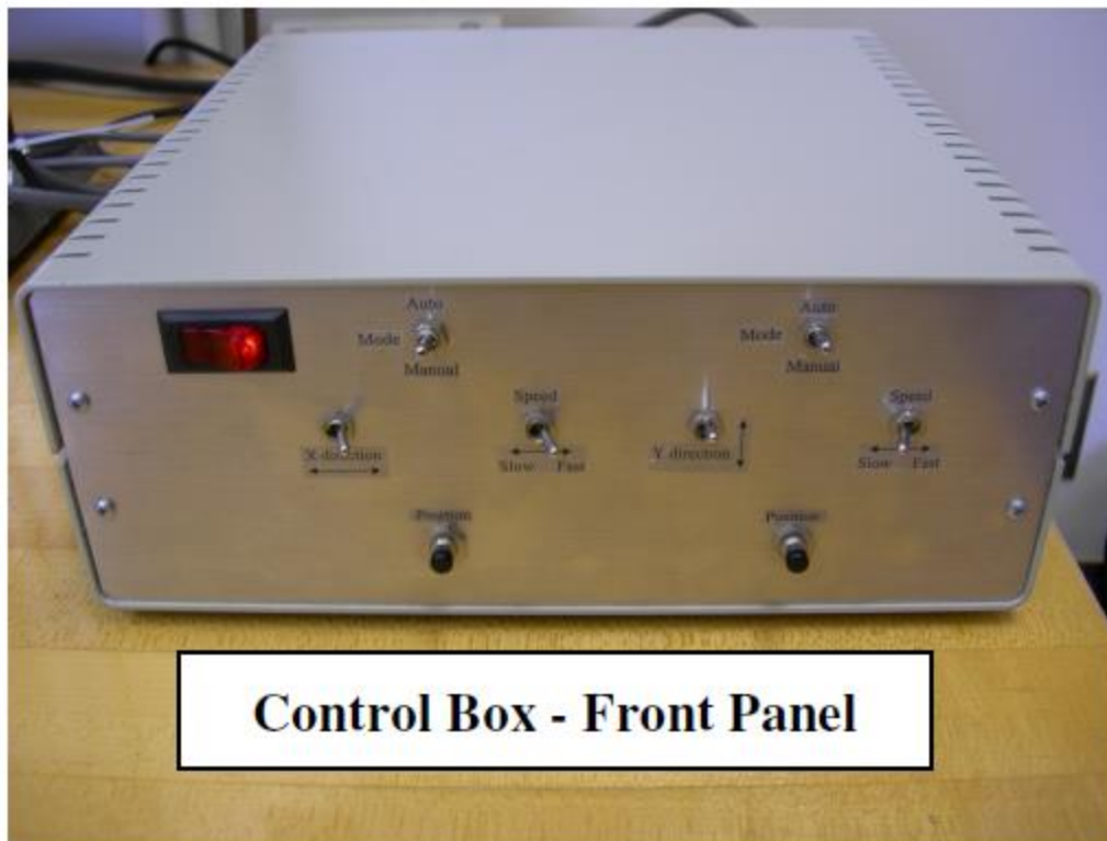
Figure 13 Control panel of surface scan profilometer (Reprinted from Malagon 2007)
