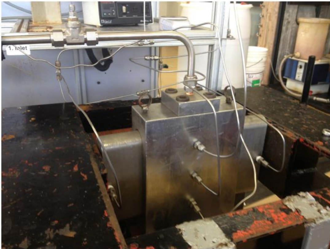
Figure 15 Acid injection apparatus, hydraulic jack and its connections
