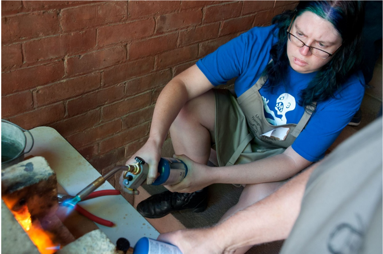
Fig. 1. A Small Forge of Cinderblocks. Photo of the author using a blowtorch with a cinderblock forge to temper steel punches at a temperature of about 1200°F. In July 2016 I took a course with Stan Nelson on “Understanding the Typographical Punch” at the Wells College Summer Book Institute in Aurora, New York, during the course of which we filed punches and created matrices for typesetting. Unpublished photograph printed with the permission of Todd Samuelson.
