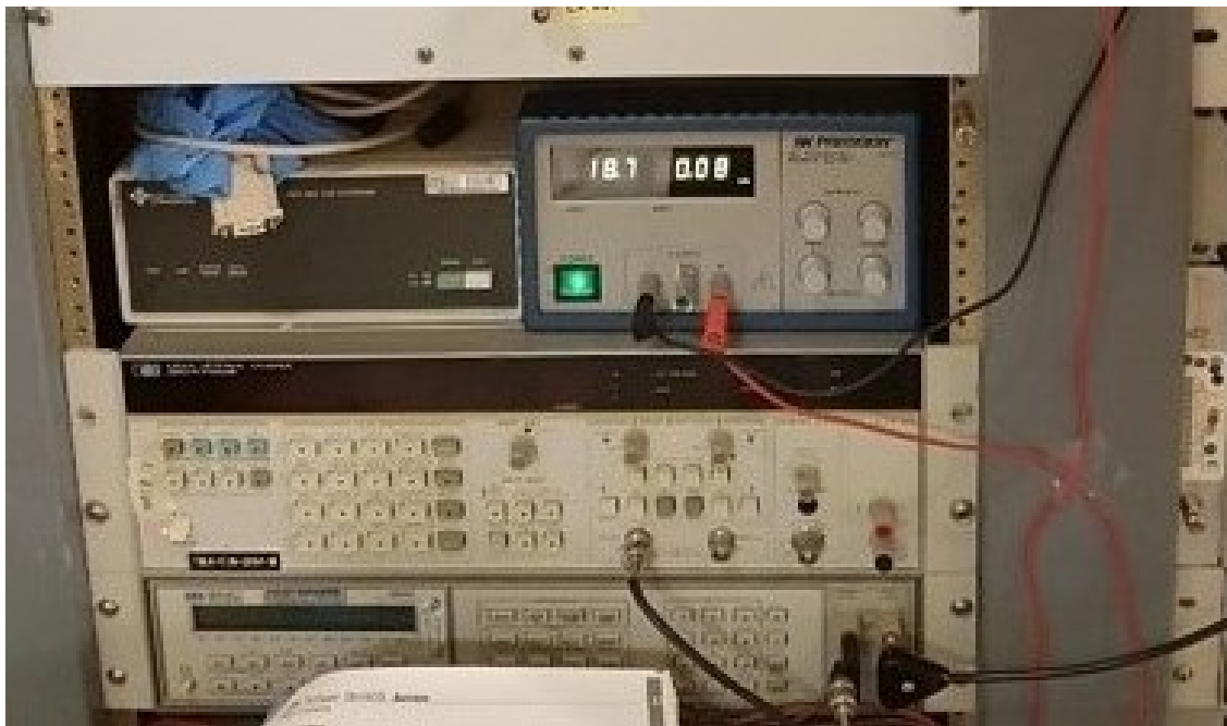
Figure 3.22: The power supply and multimeter connected to the Hall sensor
