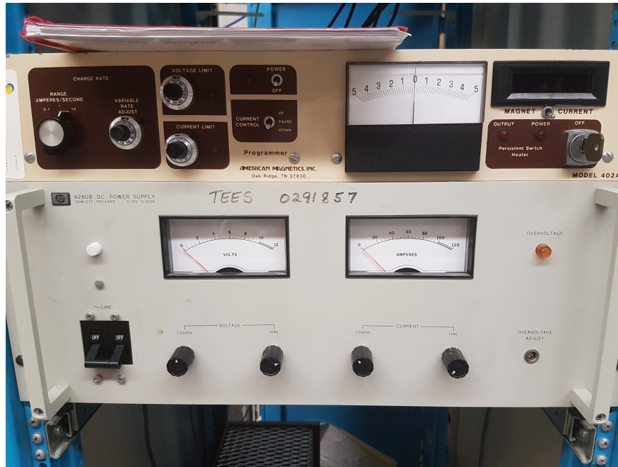
Figure 3.1: Power supply and controller for the superconducting magnet
