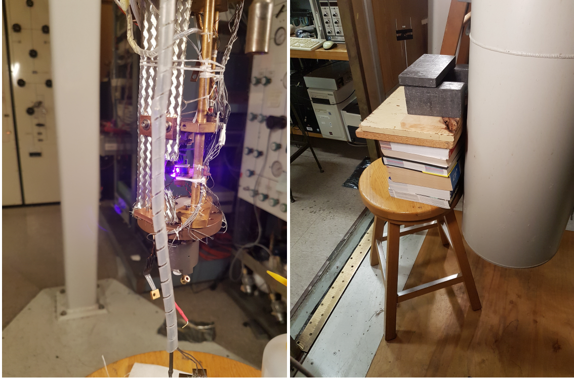
Figure 4.5: (a) The laser was used to locate the crystals. (b) Location of the Cf-252 source.
