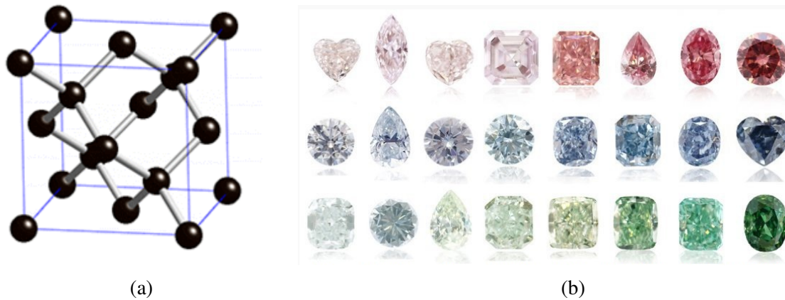
Figure 1.1: (a) The diamond lattice consists of a pair of intersecting face-centered cubic lattices, with each separated by 1/4 of the width of the unit cell in each dimension. This picture is reprinted from ref. [1]. (b) Fluorescence from different structural defects in diamond reprinted from ref. [2].
