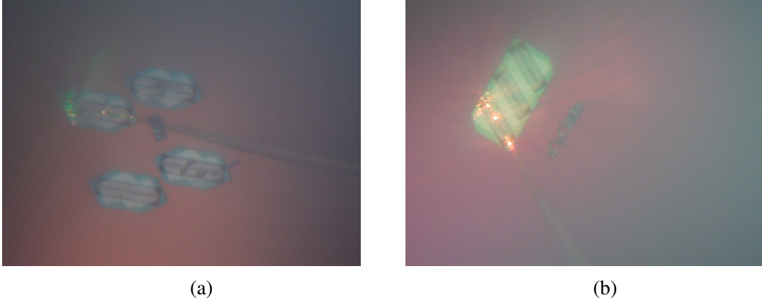
Figure 4.10: (a) Optical micrograph of an optical fiber coupled to a waveguide taper that is not appropriately rotated to the same angle of the optical fiber. (b) Optical micrograph of an optical fiber coupled to the chip behind the waveguide taper indicated by the huge scattering at the end of the taper.
