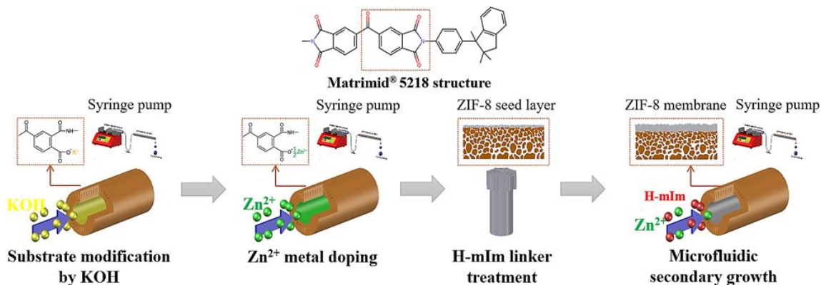
Figure 4.3 Schematic illustration of the synthesis of ZIF-8-M/HFs using combination of the PMMOF process and microfluidic secondary growth
