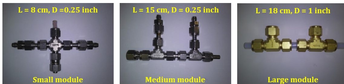
Figure 6.2 Optical photograph of different module sizes used for the synthesis of ZIF-8 membranes on polymer HFs
