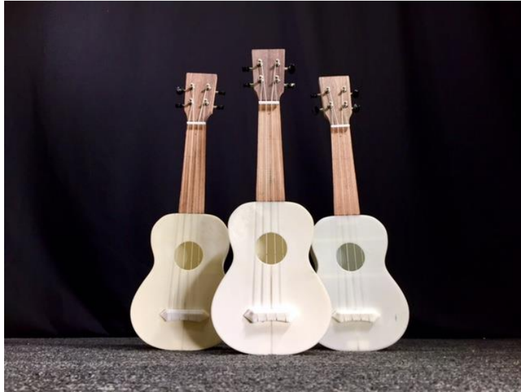
Figure 7: Printed Plastic Chamber Ukulele Specimens (ABS, PLA, HIPS)
