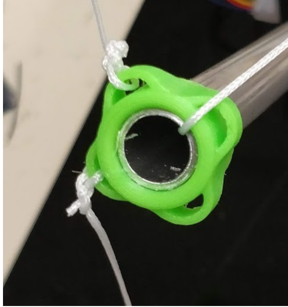
Figure 4.12: Endcap, to reduce stiction between strings and brass bar's ends.
