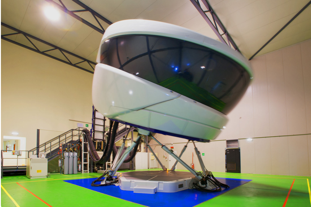
Figure 1.6: A parallel robot used as a flight simulator at SuperJet International.
