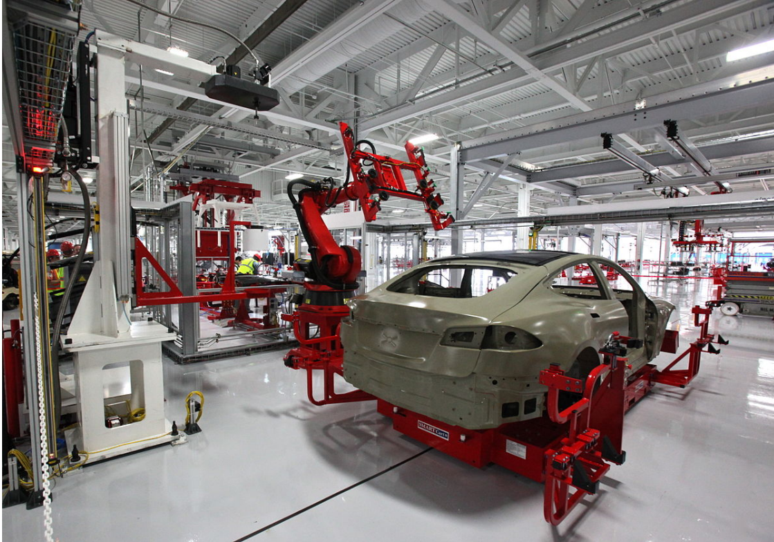
Figure 1.7: A Serial Manipulator Robot (in red) fitting Tesla S auto parts at Tesla Factory.
