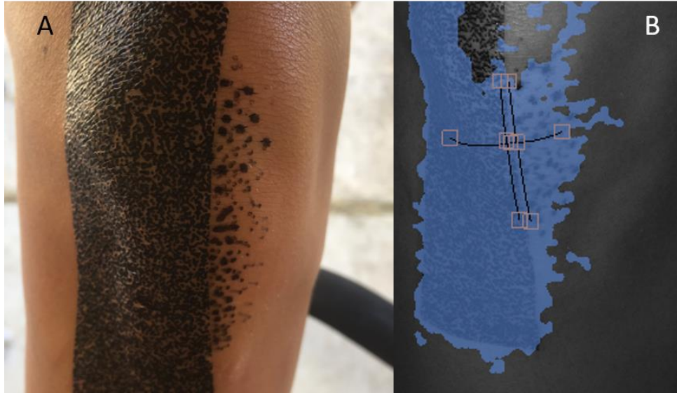
Figure 164. A) Knee with both tattoo paper and hand speckling example. B) Line gauges can be drawn in the software and data specifically from those lines can be extracted. *The blue represents identifiable facets with in the software and is used as a background to show the line gauges.
