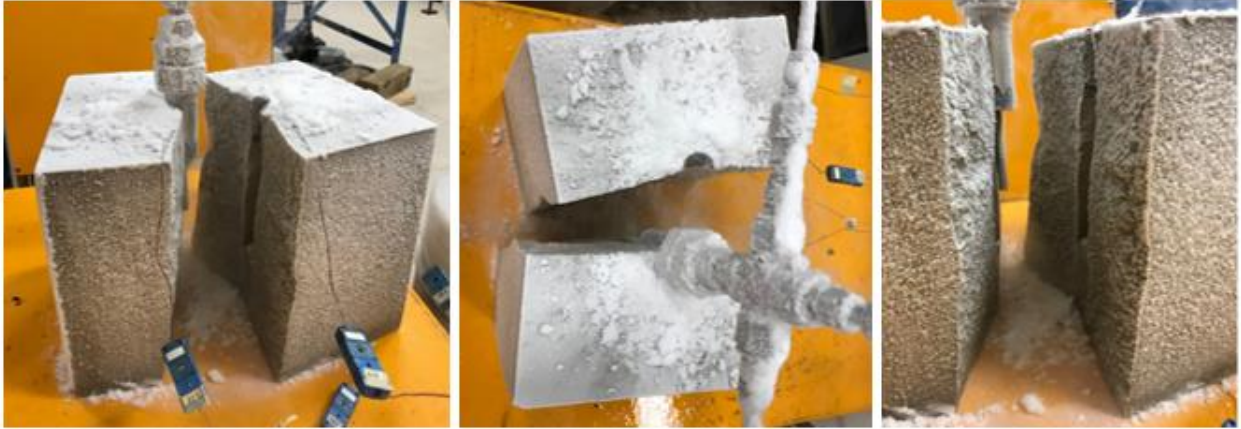
Figure 61: Sandstone block split in half after LN injection had stopped. The specimen was not moved before taking these photos.
