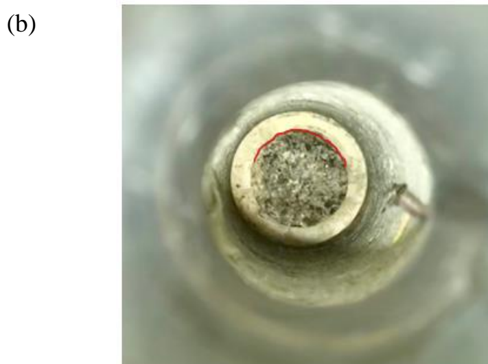
Figure 48: Con Y-9 specimen. Cracks observed after the thermal shock (a) on the surface and (b) at the bottom of the borehole.
