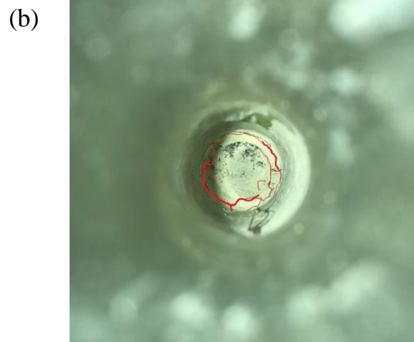
Figure 47: Con Y-10 specimen. Cracks observed after the thermal shock (a) on the surface and (b) at the bottom of the borehole.
