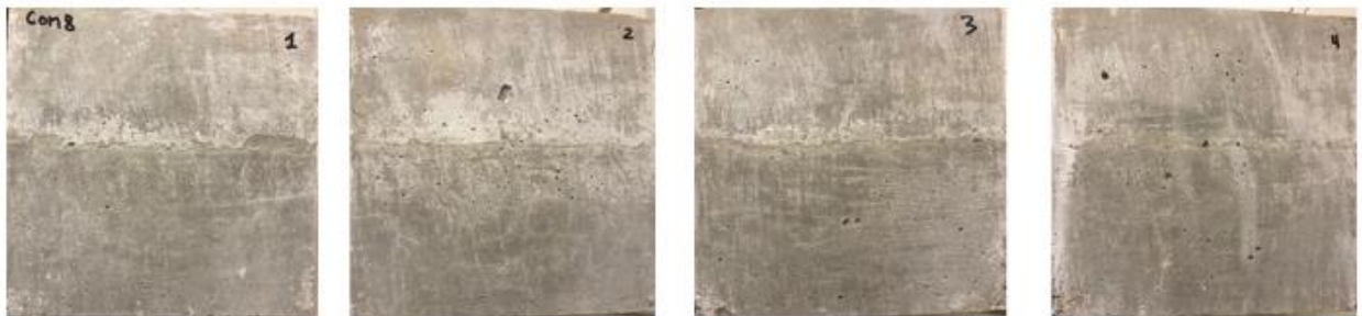
Figure 42: Con 8 weakness line. Note the visible boundary where the concrete mold was filled halfway, and thermocouples were inserted.
