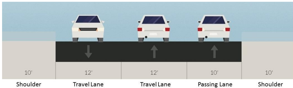
Figure 11: Proposed Arterial Road Cross-Section with Passing Lane (Super 2 configuration) for Northbound Traffic
