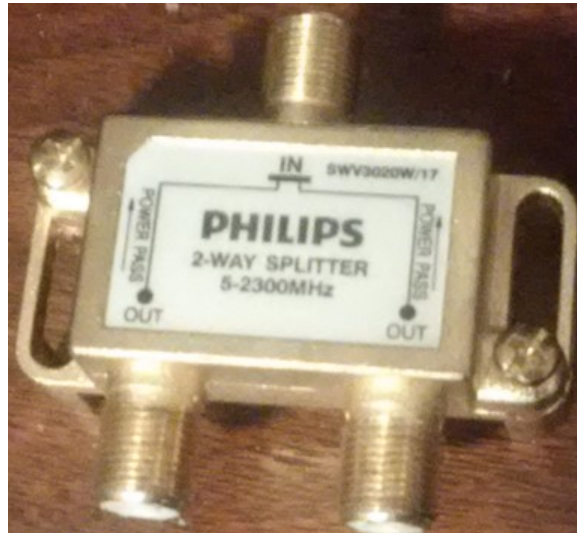
Fig. 9. An industry fabricated 3dB cable TV signal splitter. Photo taken by the author.
